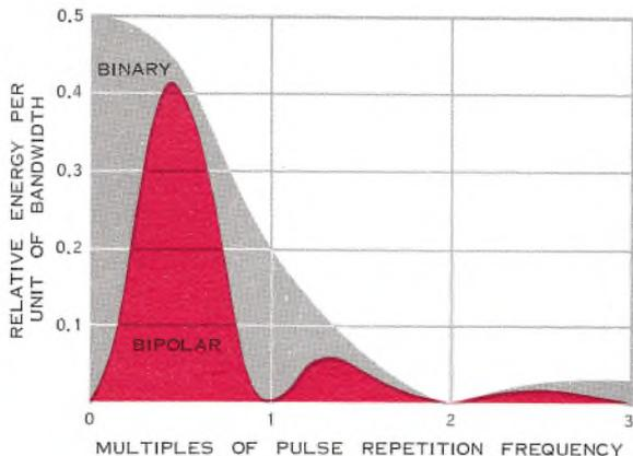
Figure 6. Energy distribution of binary and bipolar signals for 50% duty cycle pulses. Binary signal has strong discrete component at the pulse repetition frequency. Bipolar signal has no frequency components at dc or at the pulse repetition frequency; most energy falls near half the pulse rate frequency.
