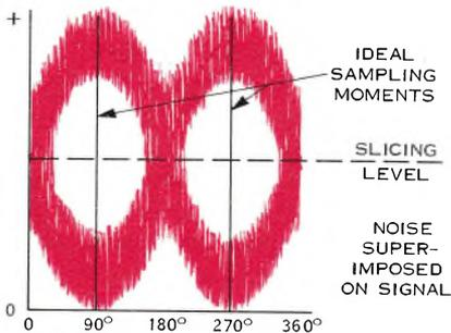
Figure 5. Shaped pulses assume sine-wave form. Noise superimposed on the waveform tends to obscure actual signal value. Timing errors can result in non-optimum sampling; increase vulnerability to crosstalk and noise.
