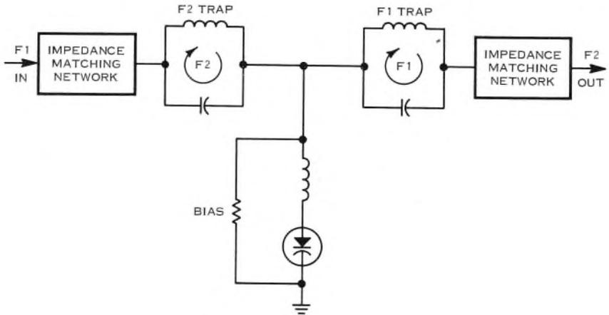
Figure 6. Typical varactor frequency doubler circuit. Frequency  $F$  is coupled to diode by series resonance of diode, inductor, and  $2F$  frequency trap elements. The  $2F$  harmonic is coupled efficiently to output, but blocked from input by trap.
