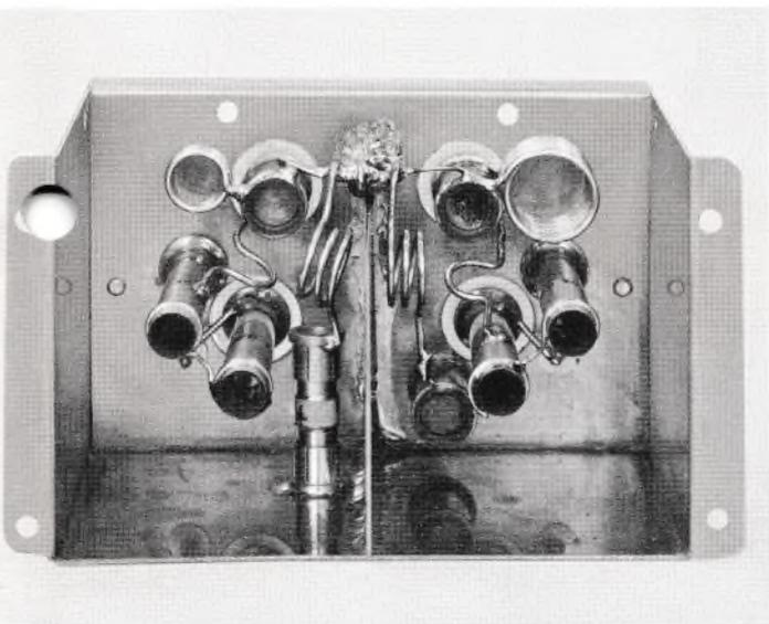
*Figure 9. Detailed view of the quadrupler. Varactor is the cylinder attached to the wall in the left chamber. Sole source of power for such circuits is the input signal. Many such stages, plus special tuners may be required to reach microwave frequencies.*
