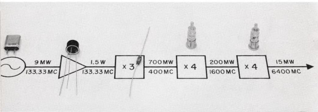
Figure 10. Simplified block diagram of an experimental microwave local oscillator. Actual circuit is much more complex than indicated here. At microwave frequencies, coaxial or stripline circuits are required. Greater multiplying factors may be achieved in each stage, but these tend to be less efficient than low-order multipliers. Principal advantage is to reduce the number of expensive diodes and other components required.
