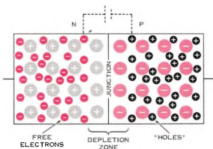
*Figure 3. P-n junction consists of semiconductor material which has been suitably "doped" with donor atoms. Field from charged donors extends across junction to repulse similarly charged current carriers (electrons and "holes"). Simulated battery represents the "contact potential" which must be overcome before current can flow. Current carriers act as capacitor plates, depletion zone serves as dielectric.*
