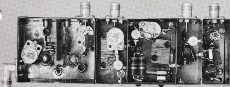
*Figure 11. Typical solid-state multiplier circuit. This "breadboard" device employs crystal oscillator to drive varactor multipliers. Output is 450-mc signal which is used to drive more multipliers.*
