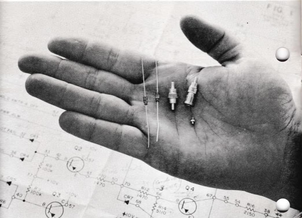
*Figure 1. Varactor diodes take many forms, of which only a few are shown here. Diodes with leads are for low frequency circuits using "lumped" circuit elements. The tiny "pill" diode is used with stripline or waveguide circuits at very high frequencies. The cartridge types may be used for all frequencies, in both lumped-element or waveguide multipliers.*
