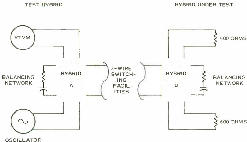
Figure 4. Typical test arrangement for measuring echo return loss. ERL measurement here depends primarily on the quality of the termination which Hybrid B provides for the two-wire line.
