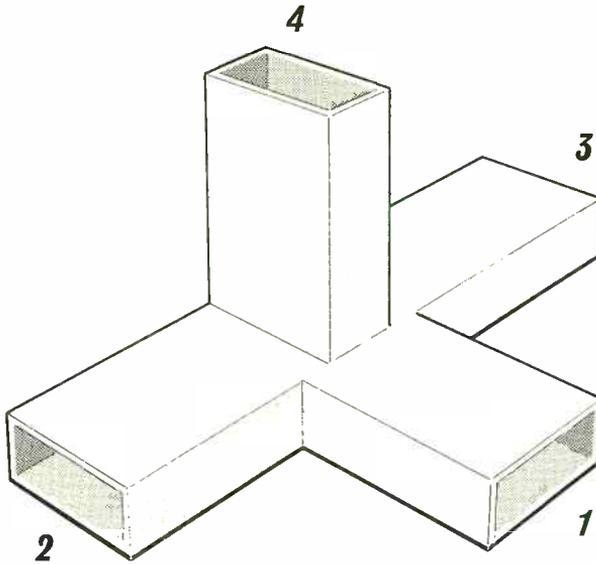
*Figure 8. "Hybrid tee," used for microwave frequencies, provides isolation between opposite arms, but maintains low-loss path between adjacent arms. A signal in arm 4 produces equal and opposite signals in arms 2 and 3, nothing in arm 1. With input to arm 1, equal in-phase signals exist in arms 2 and 3, with no coupling to arm 4.*
