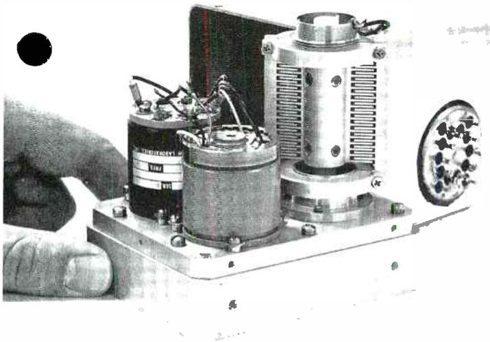
*Figure 5. Mechanical action in 27A timing system is provided by motor (left) which drives phase resolver and variable capacitor. Phase resolver follows short-term variations in data rate, while capacitor permits oscillator frequency adjustment up to plus or minus 20 parts per million.*
