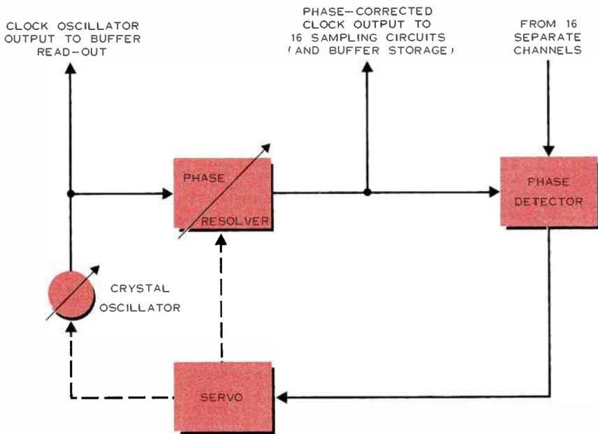
Figure 4. Simplified block diagram of timing system used in Lenkurt's Type 27A Data Terminal. Dotted lines indicate mechanical links from servo to phase resolver and oscillator.
