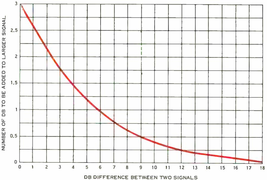
Figure 4. Addition of powers expressed in logarithmic units is simplified by the use of curve.
