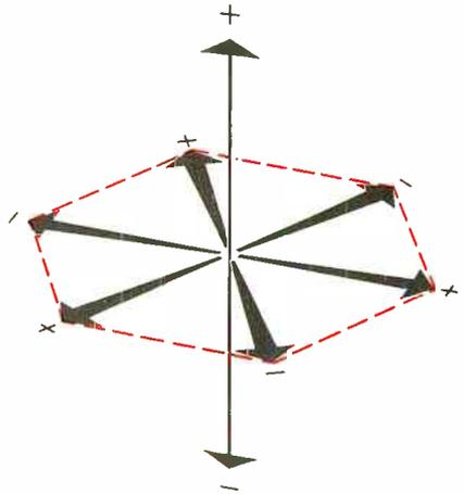
Figure 4. Crystallographic axes of the trigonal crystal system.
