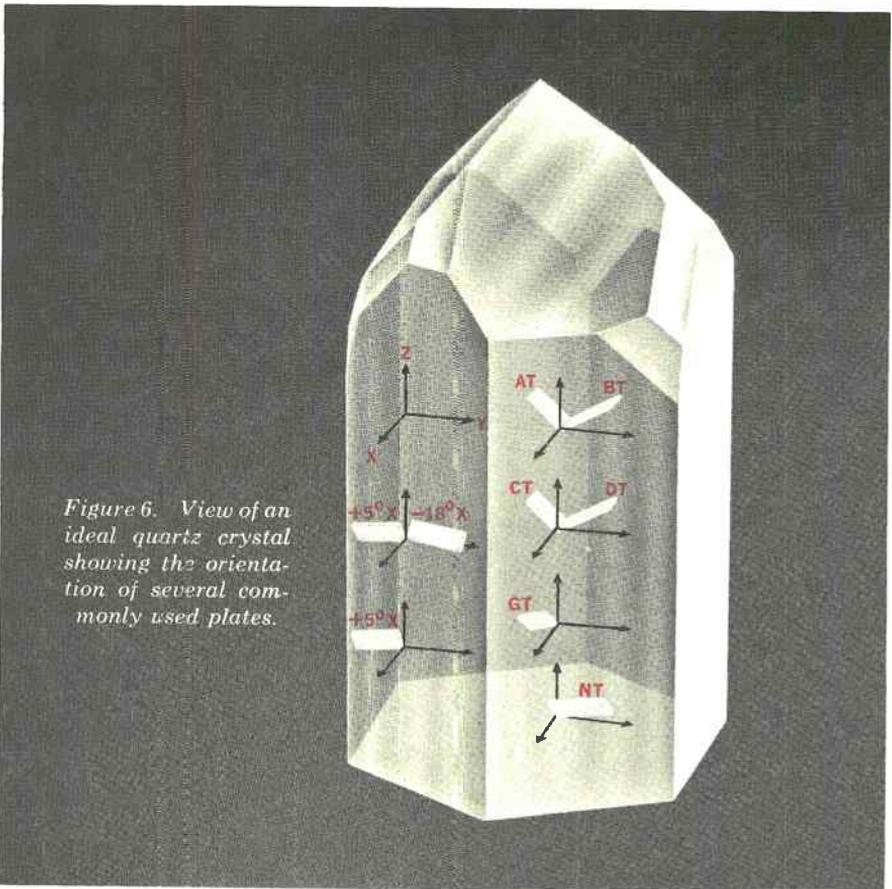
Figure 6. View of an ideal quartz crystal showing the orientation of several commonly used plates.
