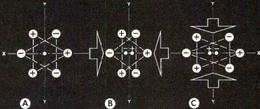
*Figure 3. A model of one molecule of a quartz crystal showing the distribution of charges. When a longitudinal force is applied a charge separation occurs along the X axis. The charge appears along the Y axis if the crystal is subjected to a shearing force.*
