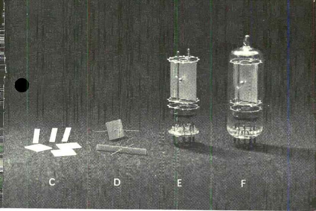
One advantage of the ceramic disc is its characteristic bandwidth, which is about 10 times larger than the bandwidth of quartz crystals. However, its Q is limited to below 2000 and its frequency stability to about 0.1 percent variation (as opposed to about 0.01 percent for quartz crystals). It is doubtful, therefore, that these devices will compete seriously with quartz crystals
