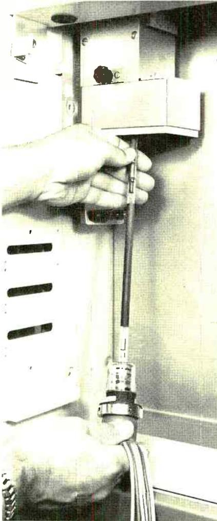
*Figure 3. Traveling-wave tube (TWT), shown here being withdrawn from its mount, acts as output amplifier for heterodyne repeater.*
