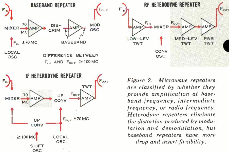
Figure 2. Microwave repeaters are classified by whether they provide amplification at base-band frequency, intermediate frequency, or radio frequency. Heterodyne repeaters eliminate the distortion produced by modulation and demodulation, but baseband repeaters have more drop and insert flexibility.
