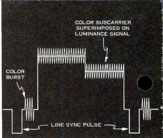
Figure 1. In the American and Canadian (NTSC) color system, "color burst" is transmitted as phase reference for color subcarrier superimposed on luminance signal. Any change in phase or amplitude of subcarrier causes color change in picture. This is called "differential phase" or "differential gain" when caused by change in luminance signal.
