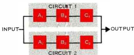
Using the formula for computing the probability function of a parallel (redundant) circuit, the overall reliability becomes:
