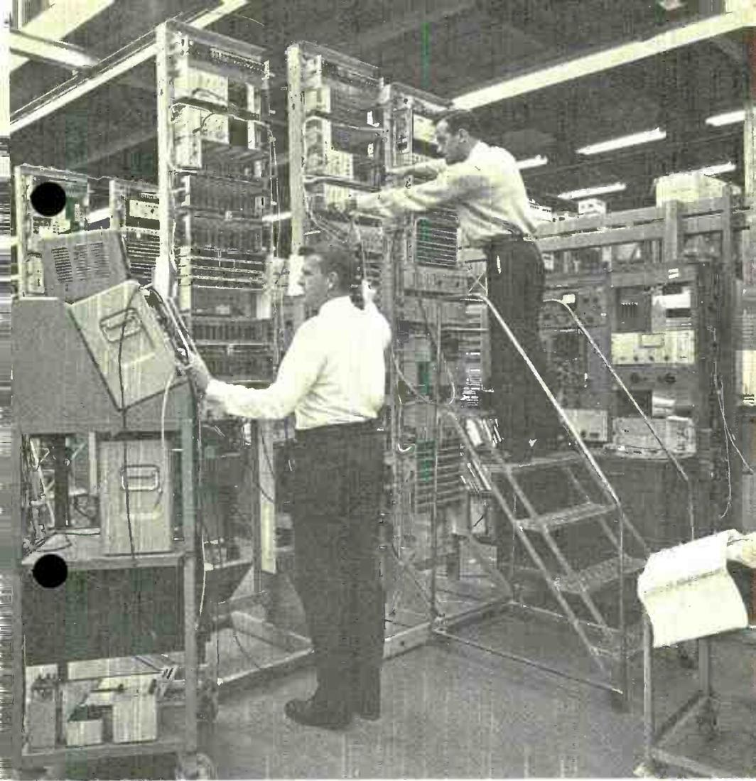
*Figure 1. Quality assurance engineers perform complete system performance test on Type 46A carrier equipment, before shipment to customer.*
