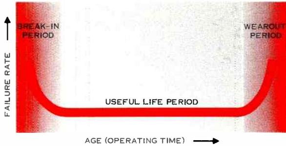
Therefore, the larger the value of MTBF the greater the reliability and, inversely, the smaller the value of the failure rate, the greater the reliability.
