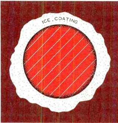
Figure 4. Current flow in a conductor covered with ice. Dot distribution indicates density of current flow.
