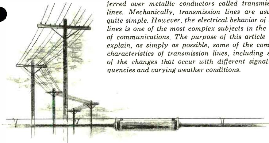
One of the most important elements in any communications system is the *transmission line* whose function is to transfer signals from one part of the system to another. The simplest transmission line consists of two parallel wire conductors with a power source at one end and a load at the opposite
