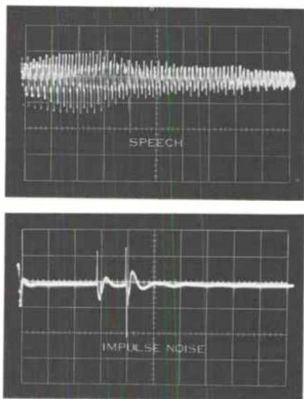
*Figure 2. Comparison of speech and impulse noise recorded from actual telephone circuit. Speech sample is the word "two." Note slight ringing following each noise impulse.*
