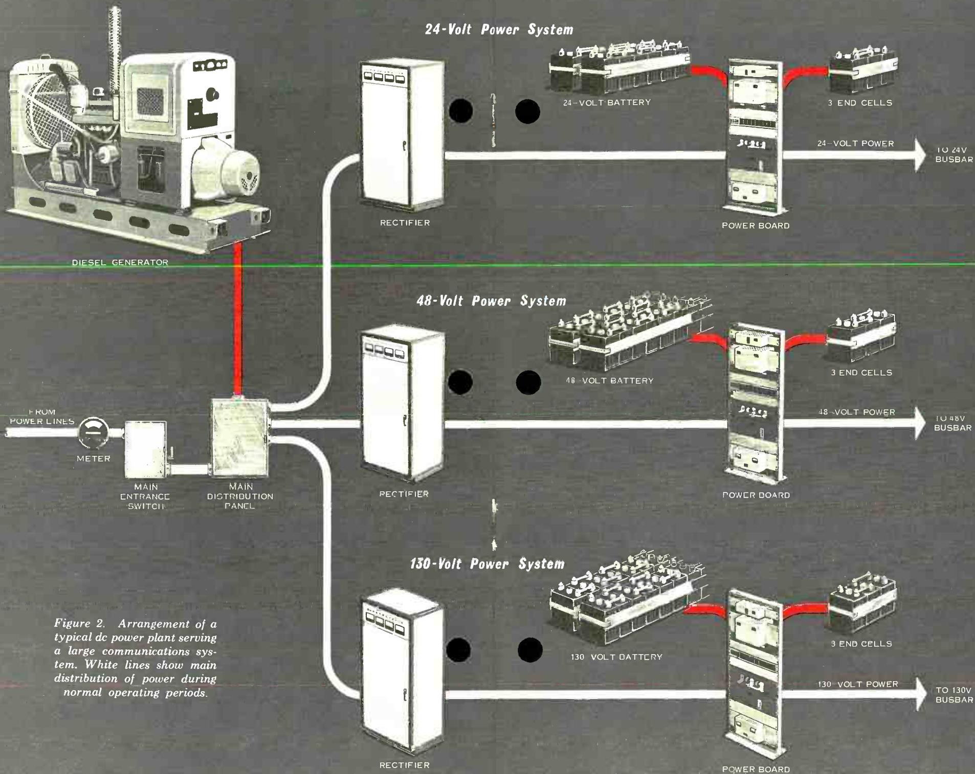
Figure 2. Arrangement of a typical dc power plant serving a large communications system. White lines show main distribution of power during normal operating periods.
