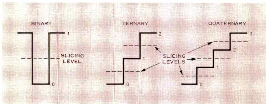
Figure 6. Multilevel codes such as ternary and quaternary increase the information capacity of the signal. However, when the peak-to-peak amplitude is the same as for a binary signal the margin against noise is reduced.
