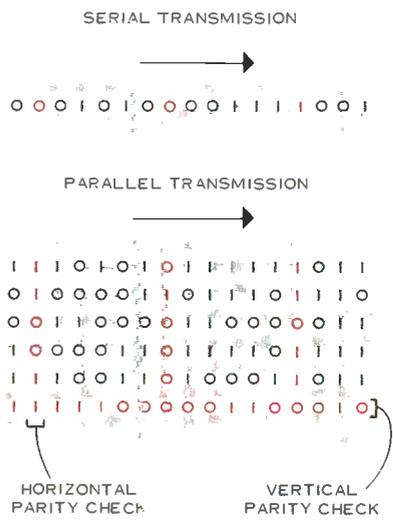
Figure 8. Typical parity checks for serial and parallel transmission. Check digit is chosen so that sum of marks in each block is always even (or odd) — wrong count reveals error.
