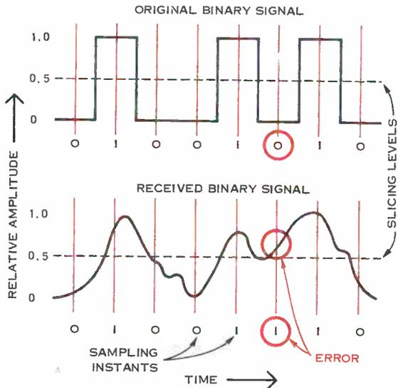
Figure 4. In a binary system, digital codes 1 and 0 are represented by different amplitude levels. When a pulse is sampled at the detector, its amplitude is proportional to the vector sum of the signal power and the noise power. The addition of this noise may distort the signal to such a degree that the detector will indicate the wrong code at the time of sampling.
