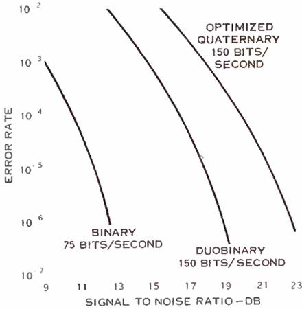
Figure 5. Error rates versus signal-to-noise ratio for three different types of digital systems.
