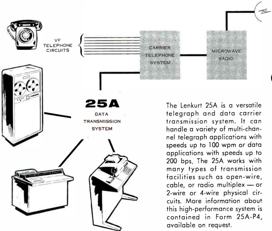
The Lenkurt 25A is a versatile telegraph and data carrier transmission system. It can handle a variety of multi-channel telegraph applications with speeds up to 100 wpm or data applications with speeds up to 200 bps. The 25A works with many types of transmission facilities such as open-wire, cable, or radio multiplex — or 2-wire or 4-wire physical circuits. More information about this high-performance system is contained in Form 25A-P4, available on request.
