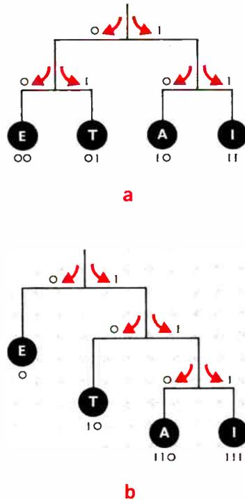
Figure 3. Two methods of coding information. In (a), characters are equally probable and two bits are required for each. In (b), characters known to appear more frequently are assigned a shorter code thus reducing the total number of bits required.
