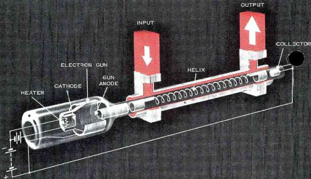
Figure 1. Construction of a typical traveling wave tube, showing the electron gun, the helix, and the collector.
