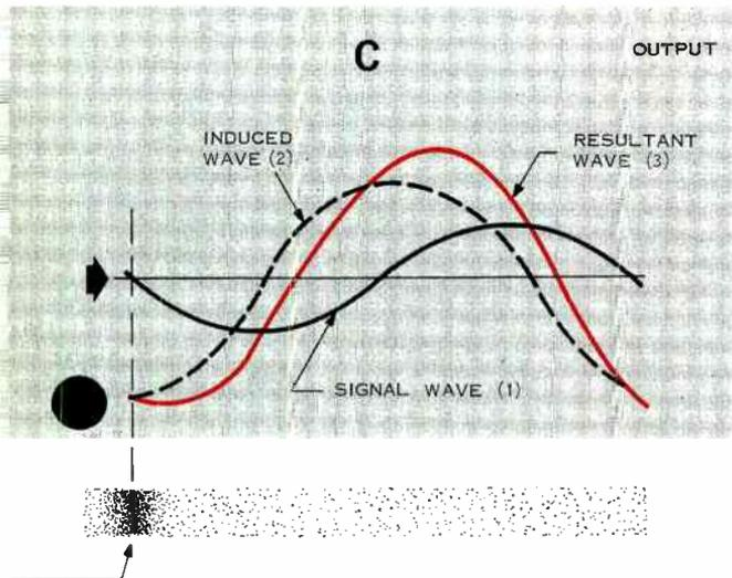
Figure 3. As the signal wave travels down the tube, electron bunches induce a second wave on the helix. The resultant of the signal wave and the growing induced wave increases exponentially.
