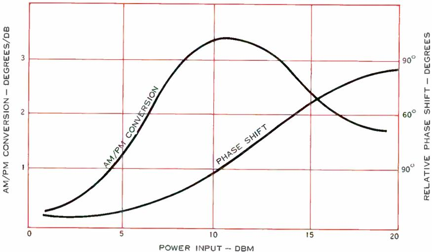
Figure 9. RF signal level vs. phase shift.
