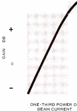
Figure 7. Gain vs. beam current.
