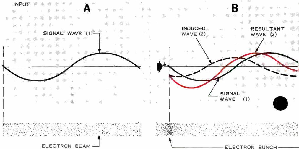
anode. As they leave the anode, the density of the electrons is uniform. The beam electrons are accelerated, by a positive voltage potential on the helix, to a velocity  $U_0$ , which is proportional to the square root of the helix voltage,  $V$ , as shown in the following equation.
