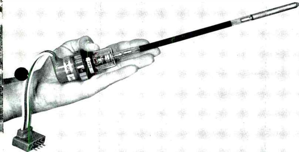
*Figure 10. Photograph of typical traveling wave tube used in a microwave heterodyne repeater system. Tube operates in the 6000 megacycle band.*
