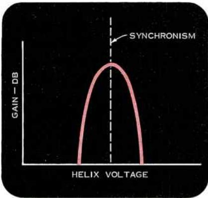
Figure 6. Gain vs. helix voltage.
