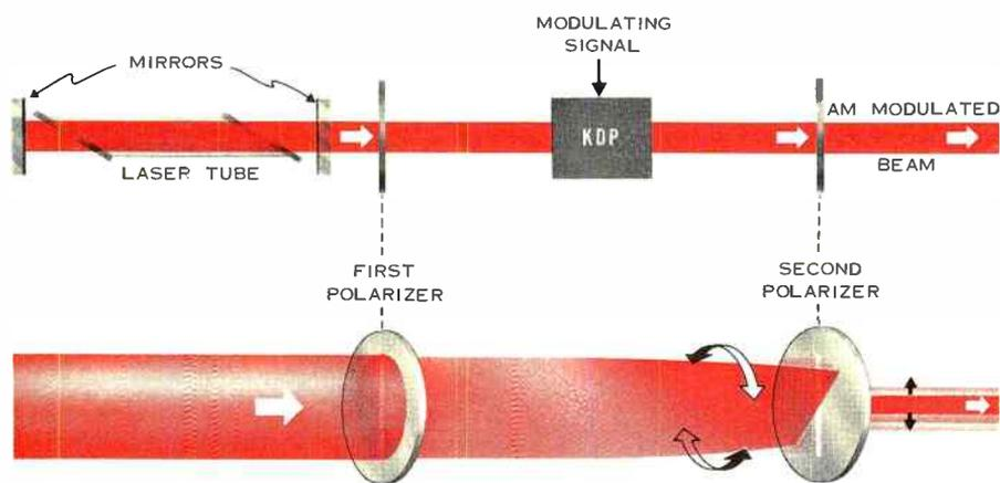
Figure 6. As beam passes through an AM laser modulator, it may be visualized as a ribbon of light twisting proportional to a signal applied to the KDP crystal.
