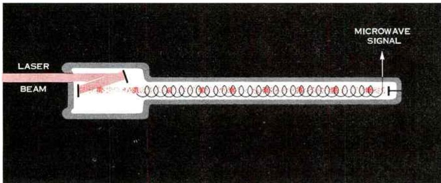
*Figure 9. The microwave phototube converts laser light to electrons, bunched proportionate to the original modulation. The current induced in the helix is then processed by usual microwave techniques.*
