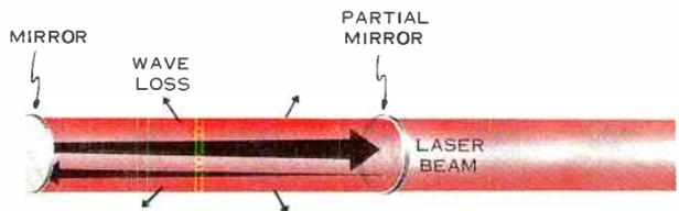
builds up standing waves which continue to multiply on each pass through the cavity. When the gain is strong enough to overcome the loss in the mirrors, an intense beam is emitted from the partially transparent mirror. As the light bounces back and forth, any waves moving at angles to the axis between the mirrors will soon leave the system through the walls of the tube. Therefore, the output beam of the laser will be extremely parallel.
