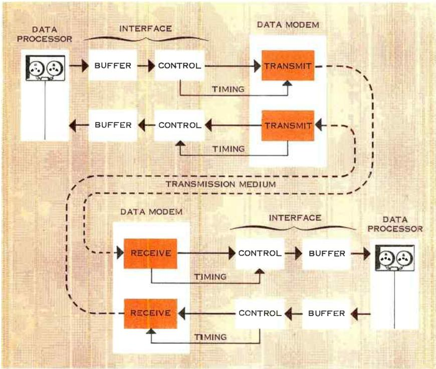
Figure 1. Typical full-duplex data transmission system arrangement. Timing signals from control unit synchronize data transmitter with data processor. At receiver, the element of time is important in reconstructing the original digital representation of the data. This is accomplished by deriving sync pulses from the data stream.
