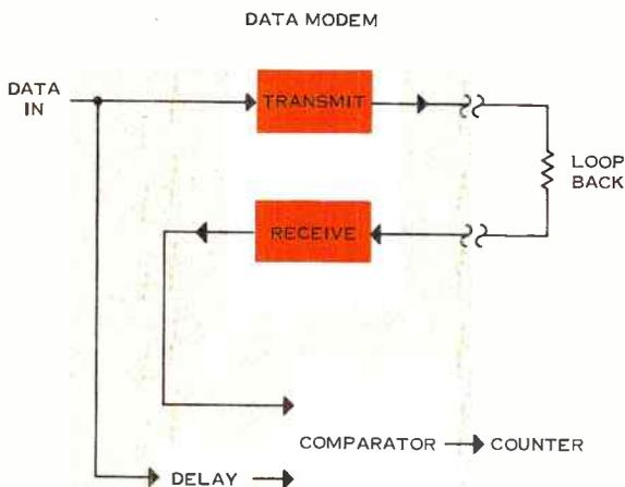
*Figure 2. Typical method for measuring error performance of a data communications set. Data signals are looped back from transmitter to receiver. Delay corresponding to the amount in the path is added to the original data signals which are then compared bit-by-bit with the received data signals. An error counter keeps track of the number of errors.*
