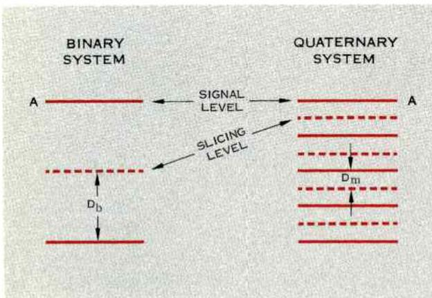
*Figure 3. Determining noise penalty compared to binary. Because multilevel systems require more slicing points than binary systems, they are more susceptible to errors caused by noise.*
