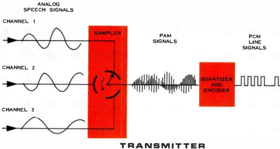
Figure 2. Simplified time division multiplex PCM system.
