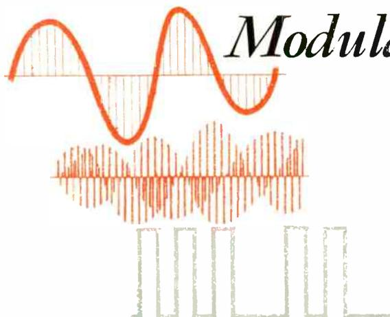
*The constant search for better communications at lower cost has led the telephone industry to a radically different method of transmitting speech information. This method, using binary digital pulses rather than conventional analog signals, provides high quality transmission and has proven to be very economical in short-haul carrier systems.*
