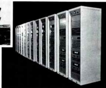
Communications between the Apollo moonship and earth will be conveyed by Lenkurt 46A multiplex equipment aboard tracking ships stationed around the world.
