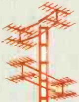
*Master antenna systems are serving an increasing number of American communities, providing television reception where before there was none. By extending the viewing area of both commercial and educational television stations, these small networks of coaxial cable and microwave radio have collectively established a new and sizeable industry.*
