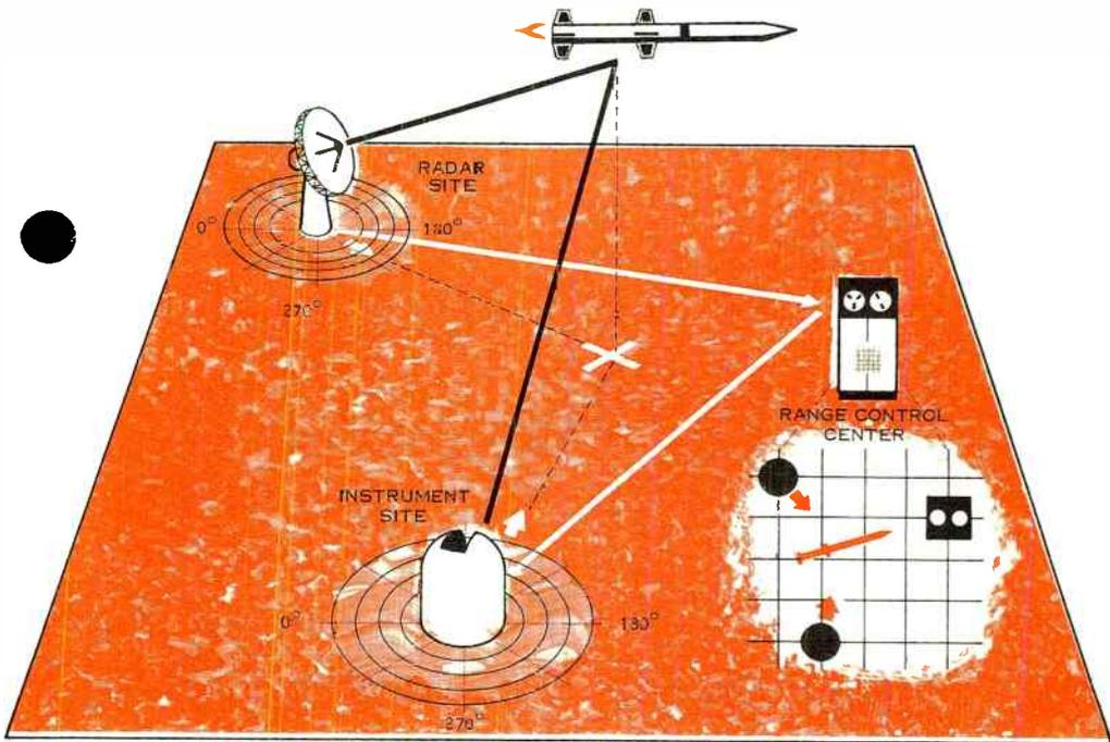
Figure 3. Radar picks up missile after launch, sends polar coordinate tracking information to the range control center. Computer translates to Cartesian system, sending pointing information to other instrument sites.
