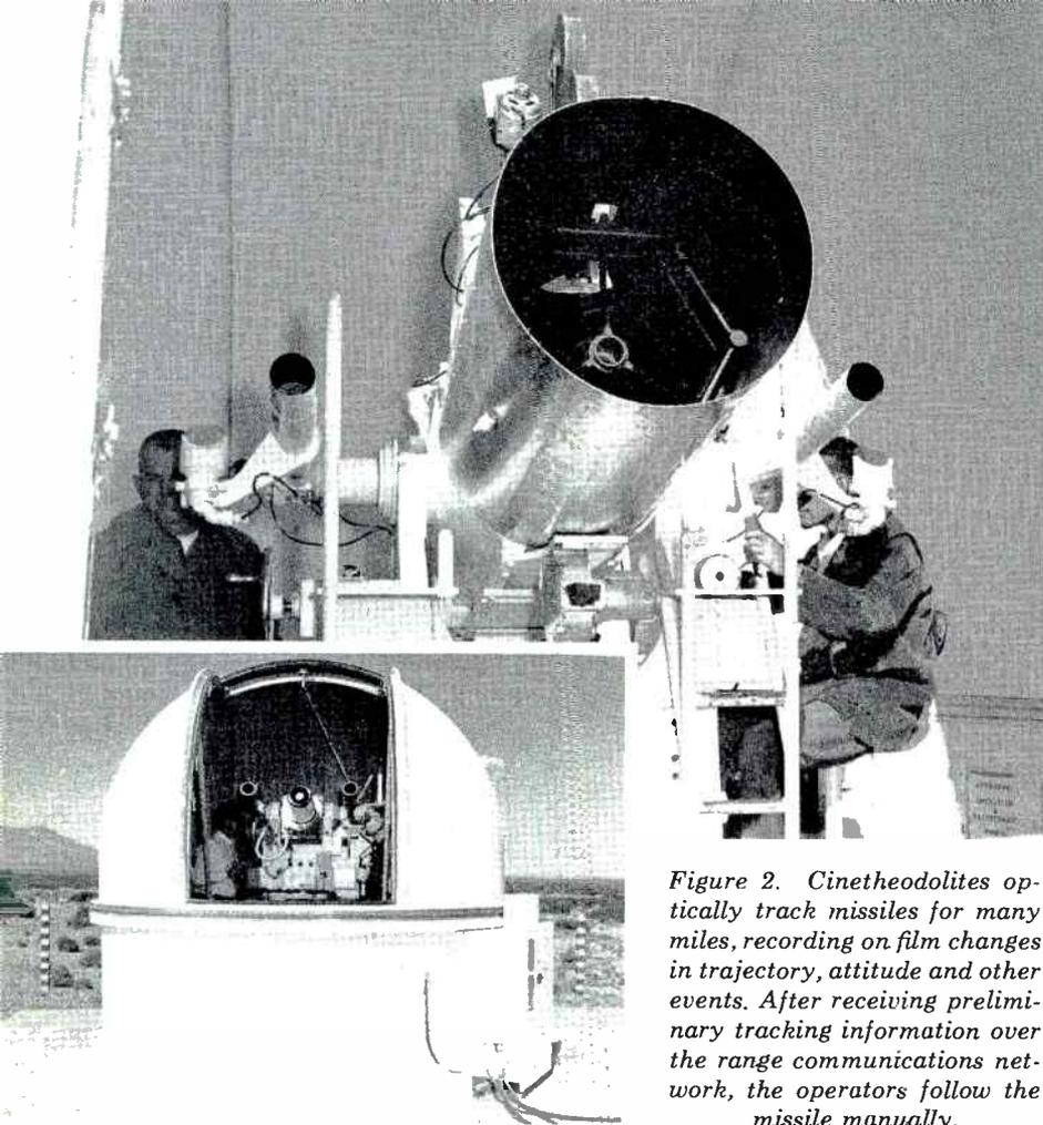
*Figure 2. Cinetheodolites optically track missiles for many miles, recording on film changes in trajectory, attitude and other events. After receiving preliminary tracking information over the range communications network, the operators follow the missile manually.*
