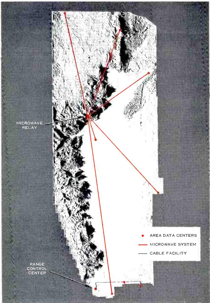
Figure 4. Microwave system recently installed at White Sands Missile Range by Lenkurt relays instrumentation and data control information between area data centers and range control center. Many instruments surround each site, linked by hard line facilities.
