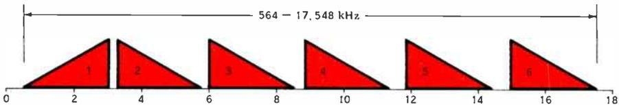
Figure 4. The modulation scheme used with the L4 combines six 600-channel mastergroups between 564 kHz and 17,548 kHz. Mastergroups 2 through 6 use the upper sideband while mastergroup 1 uses the lower sideband.
