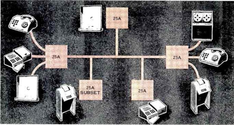
*Figure 2. The Lenkurt 25A data transmission system makes it possible to use one voice circuit for a number of data channels. The 25A operates between 75 b/s and 200 b/s with a maximum of 25 channels per voice circuit.*
