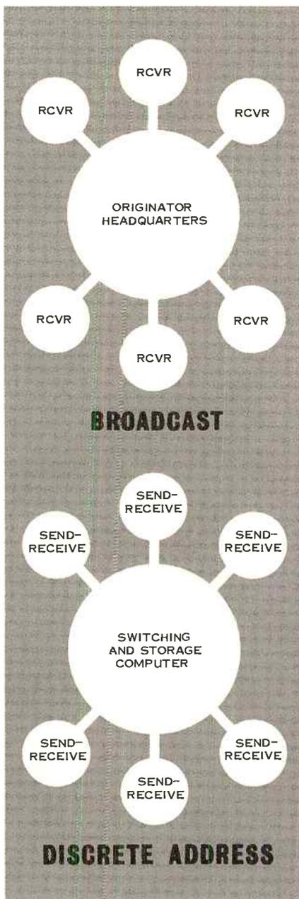
*Figure 1. Data communications systems fall into one of two general categories. One is essentially a receive-only system while the other has stations with a send and receive capability.*
