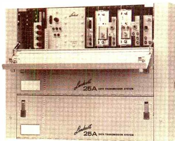
*Figure 4. The Lenkurt 25A is an economical, highly reliable data transmission system which uses sharp filtering to transmit up to 50% more information than conventional systems.*
