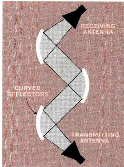
*Figure 4. Reflecting beam waveguides use optical techniques to reflect millimeter wave energy along a path. Reflectors are usually curved to focus energy and reduce spreading losses.*
