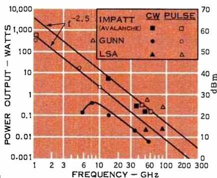
Figure 1. Maximum power produced by three solid-state devices. Note that the maximum pulsed power of the IMPATT avalanche type diode and Gunn diode decreases as frequency increases in the proportion  $f^{-2.5}$ .
