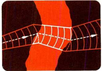
*Figure 2. An electromagnetic wave is refracted when it encounters a medium of different density. The resulting speed change usually causes a change in direction.*
