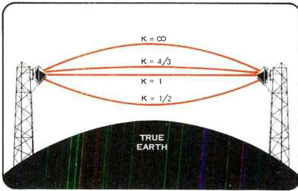
Figure 4. The equivalent earth radius factor  $K$  shows the path of a microwave beam relative to the surface of the earth. (For the purpose of illustrating this, the earth's curvature is exaggerated.)
