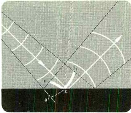
*Figure 1. An electromagnetic wave undergoes a change of direction and usually a change of phase at reflection.*
