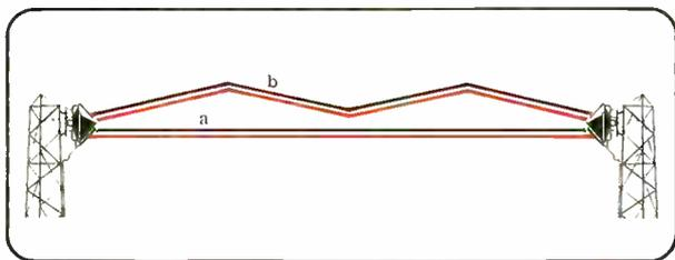
*Figure 6. With frequency diversity two wavelengths travel the same refracted path (b) but will not have the same interfering effect on the direct wave (a).*
