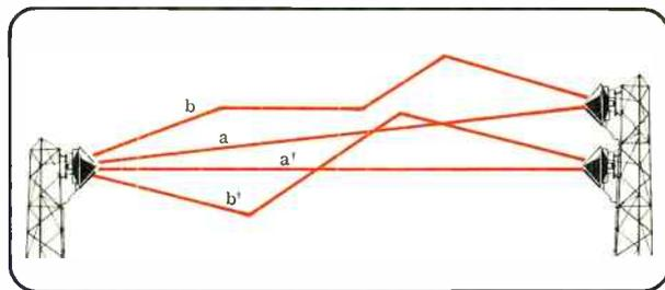
*Figure 7. With space diversity the same wavelengths travel different refracted paths (b and b') but will not have the same interfering effect on the direct waves (a and a').*
