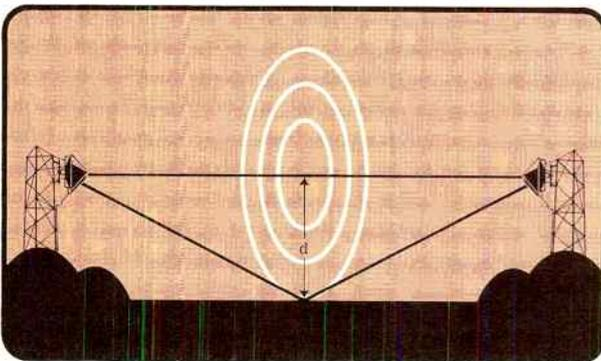
*Figure 9. Reflected waves can interfere with direct waves. A distance,  $d$ , between reflecting point and direct wave equal to an odd Fresnel zone radius can cause reinforcement. If  $d$  equals an even zone radius, the two waves can cancel.*
