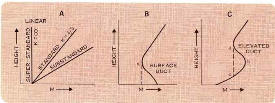
Figure 3. Typical  $M$  profiles showing atmospheric conditions. Profiles B and C indicate an inversion which can cause ducting. Each profile has associated with it different propagation characteristics.
