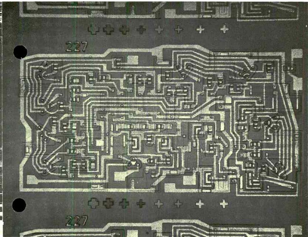
*Figure 7. Sylvania IC contains 116 transistors, resistors and diodes to produce 40 gate circuits on each chip. Used in computers or digital communications equipment.*
