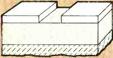
Window etched through silicon dioxide to expose epitaxial layer to diffusion.
