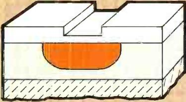
Impurity is diffused into silicon. In the process, new oxide layer forms over entire surface.
