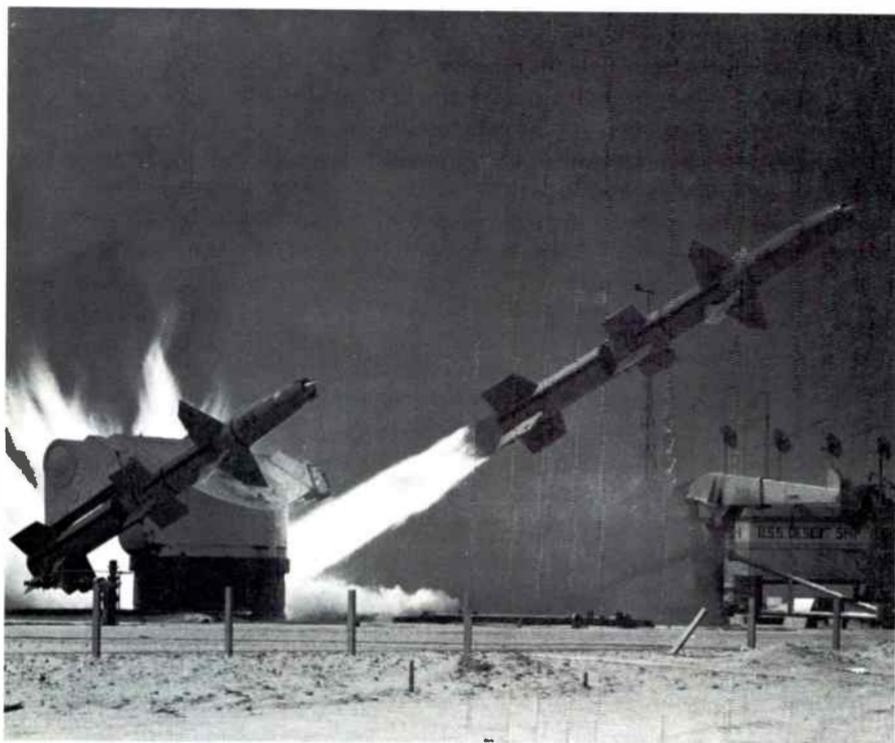
*Figure 6. Short and long range missiles must undergo the same demanding tests before they become operational. Here, the TALOS is fired from a simulated ship at White Sands. The missile is under constant surveillance as it passes over the range.*
