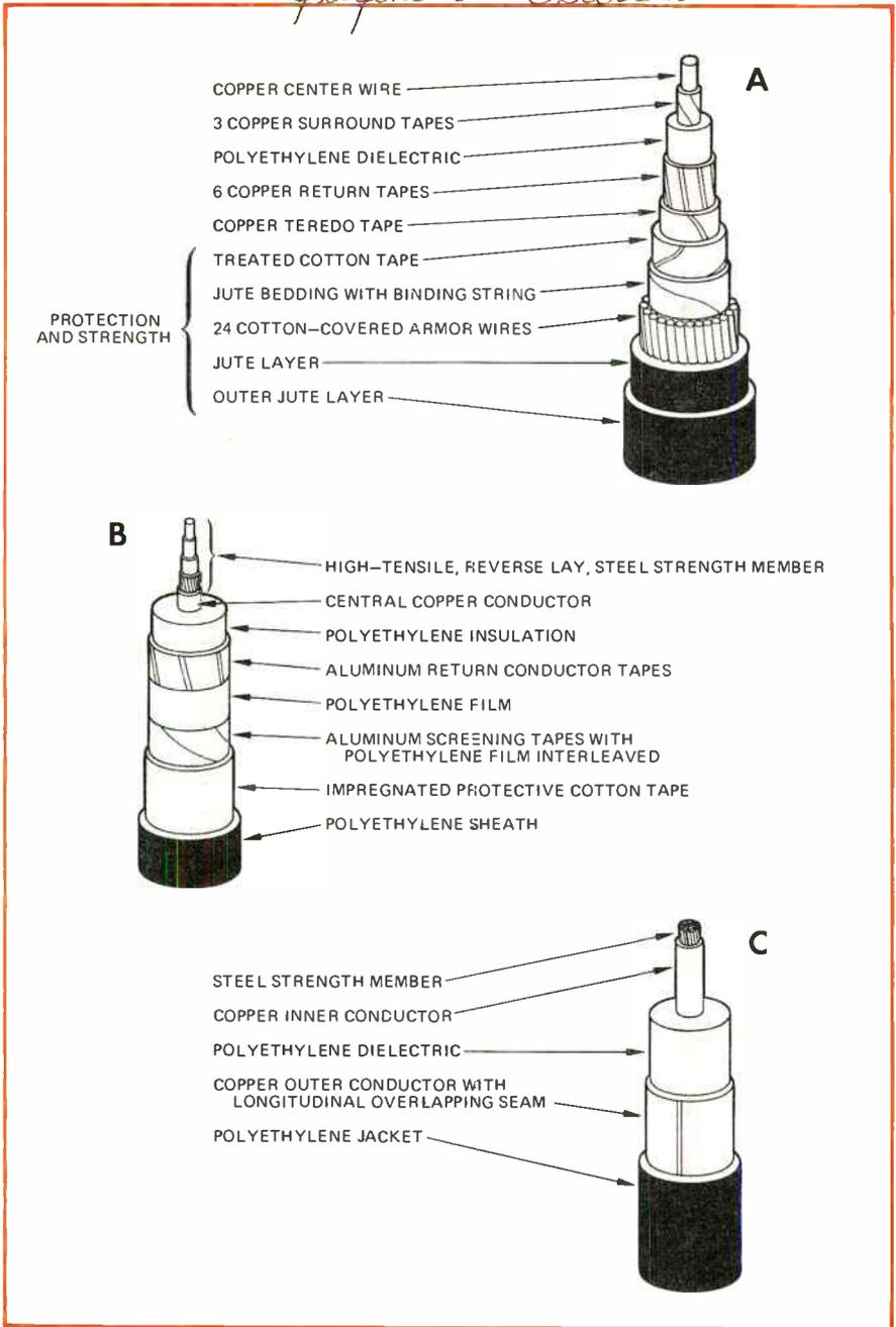
Figure 1. Armored cable shown in A was used in the SB system. B and C show armorless cable developed by the British Post Office (B) and American Telephone and Telegraph (C). All three cables measure 1-1/4 inches in diameter.
