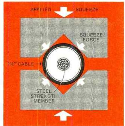
Figure 4. End view of cable engine as repeater enters engine. Insert shows how tracks grip a piece of cable. When repeater goes through, the flexible tracks separate to give the necessary clearance.
