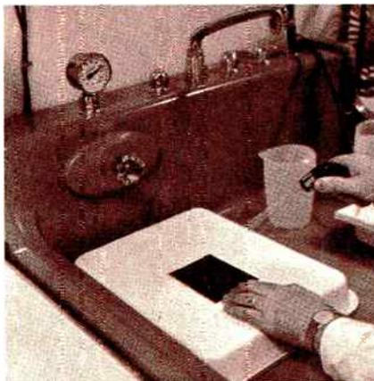
*Figure 2. The resistor pattern can be seen emerging from the stencil film as the unexposed area is rinsed away. Using the temperature blender in the background, a steady water temperature of 110° is maintained.*
