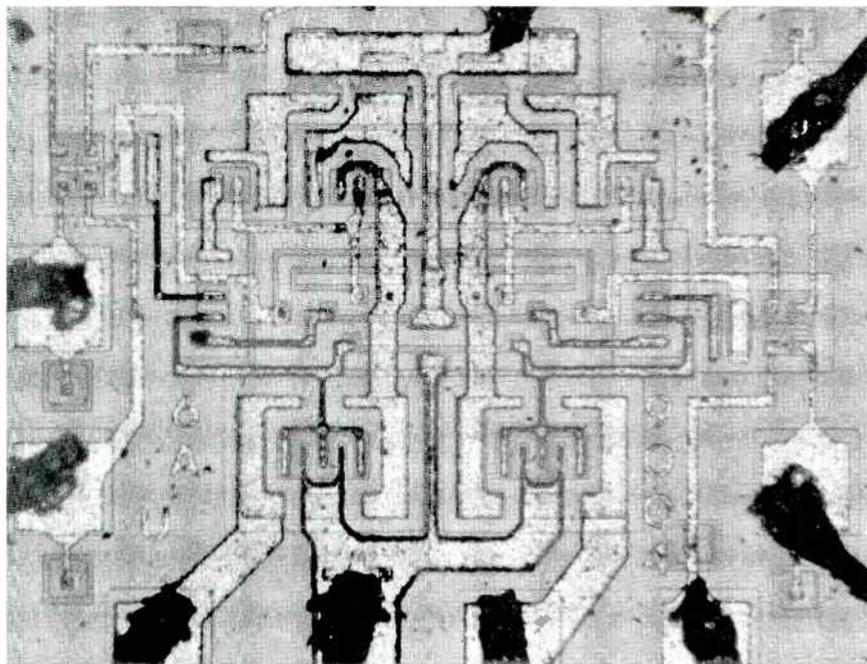
Figure 7. Also used in the 91A, this digital IC has two 4-input NAND gates.
