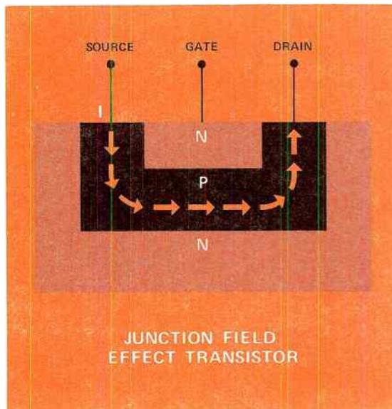
*Figure 4. Current (I) flowing in the channel is controlled by varying the voltage across the gate. The applied voltage creates a field in the channel which has a "pinching" effect on the current. Thus, channel current can range from almost zero to full conduction. Since they are voltage controlled, unipolar FET's more closely resemble vacuum tubes than do their more common cousins which are bipolar and current controlled.*
