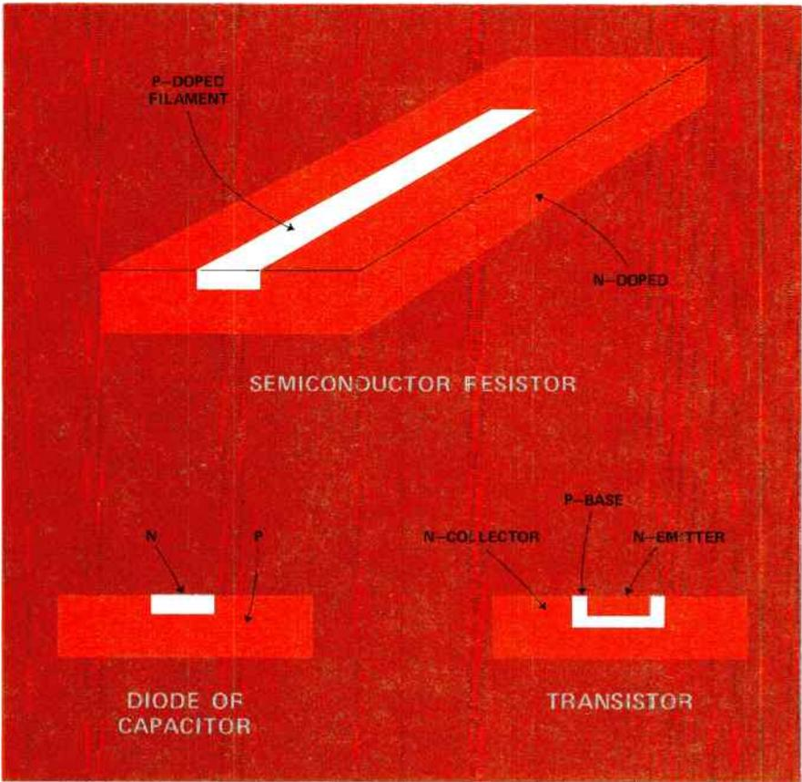
Figure 3. Semiconductor microelectronic devices
