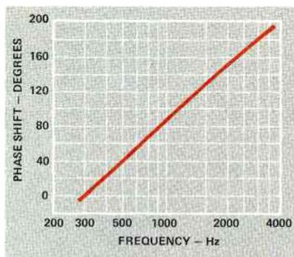
Figure 1. Cosine section phase shift-versus-frequency characteristic — Amplitude Equalizer.
