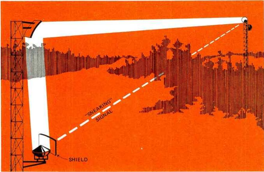
*Figure 4. In situations where the path is not effectively obstructed, the signal may sneak from the illuminating dish, directly to the distant receiver. This bypassing of the reflector causes noise at the receiver. Shielding is used to control this problem.*
