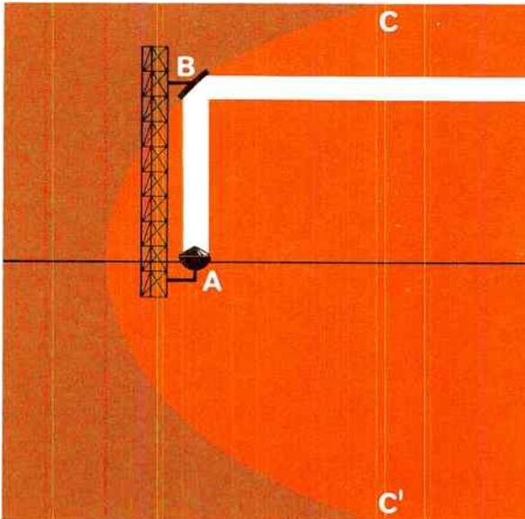
Figure 5. To calculate the curve of a periscope reflector (B), it is convenient to consider the illuminating dish (A) as the focal point of the parabola represented by  $CC'$ . The reflector (B) may simply be considered a solid segment of the imaginary parabolic shell.
