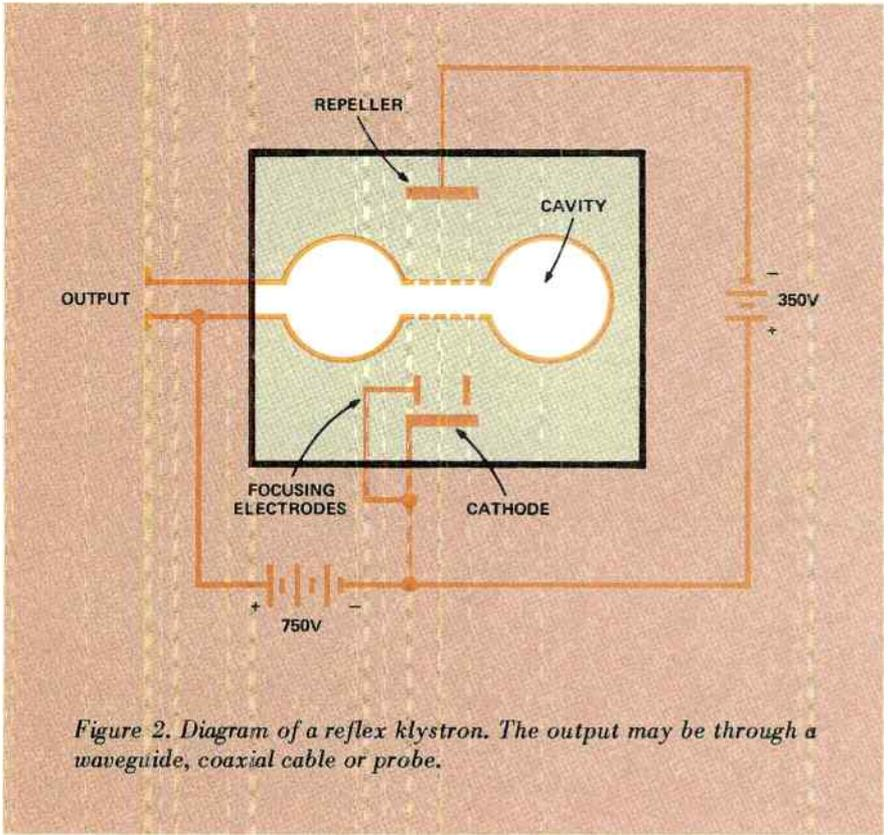
Figure 2. Diagram of a reflex klystron. The output may be through a waveguide, coaxial cable or probe.
