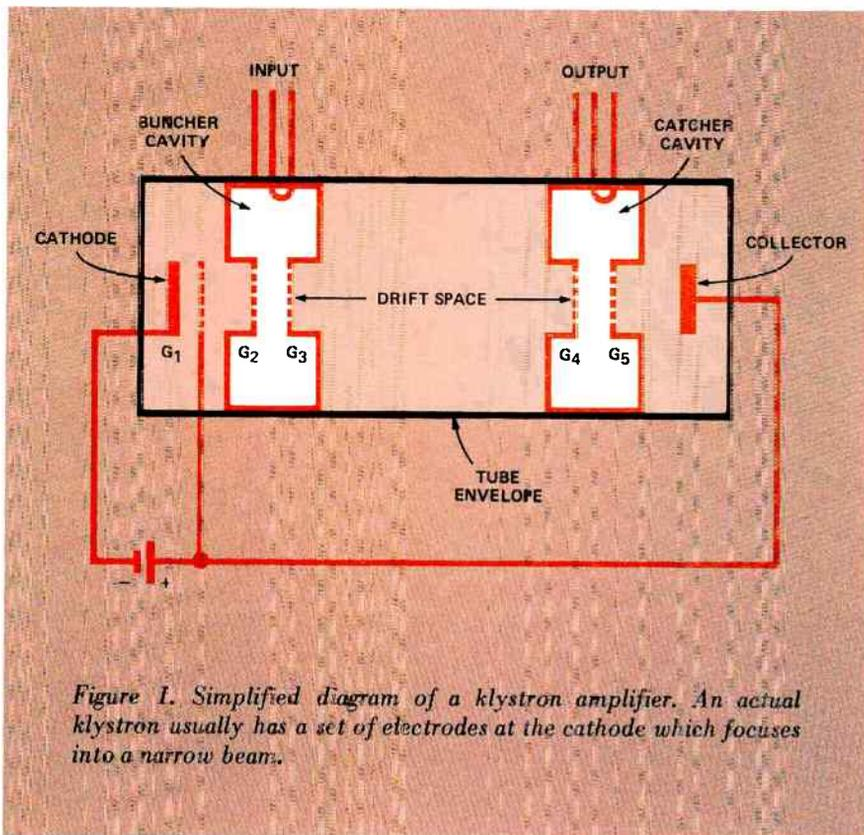
Figure 1. Simplified diagram of a klystron amplifier. An actual klystron usually has a set of electrodes at the cathode which focuses into a narrow beam.
