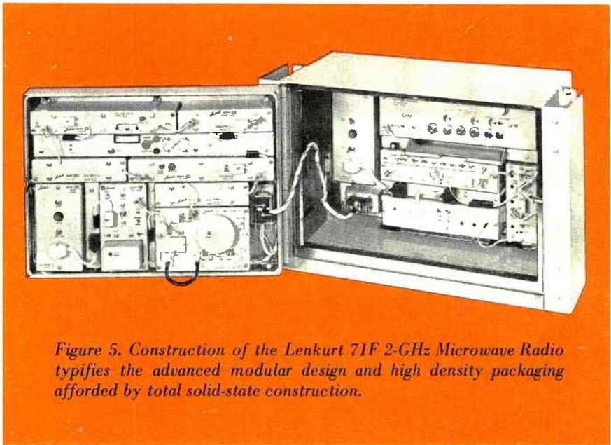
*Figure 5. Construction of the Lenkurt 71F 2-GHz Microwave Radio typifies the advanced modular design and high density packaging afforded by total solid-state construction.*
