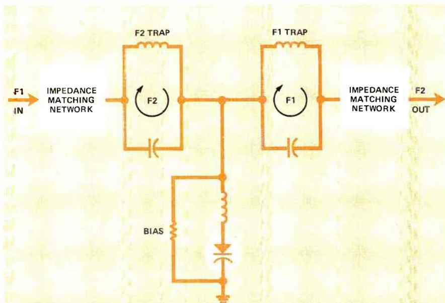
*Figure 4. This greatly simplified schematic represents multiplier's typically found in solid-state microwave radios. A six-stage multiplier would use three such circuits, a twelve-stage, six and so on.*
