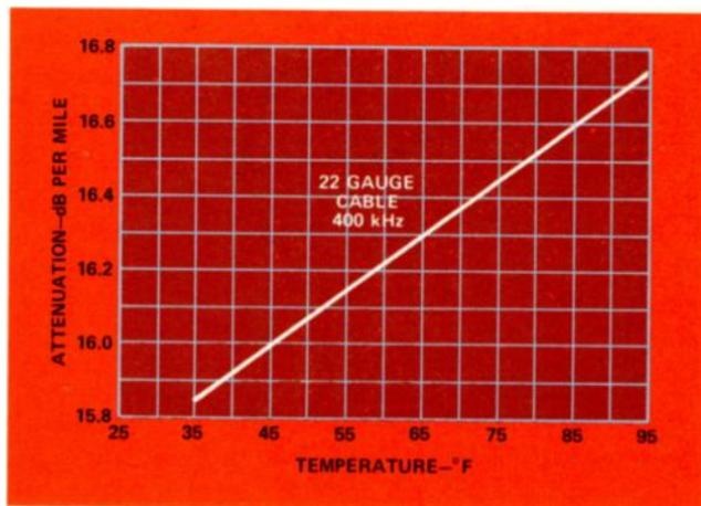
Buried cable is thermally insulated by the earth, and its year-round temperature variation in some areas will be no more than a few degrees. Aerial cable, with no such insulation, suffers from an "oven effect" that exaggerates the sun's heat. Tests have shown that the internal temperature of aerial cable on a hot day may be 18 degrees higher than the ambient air temperature.
