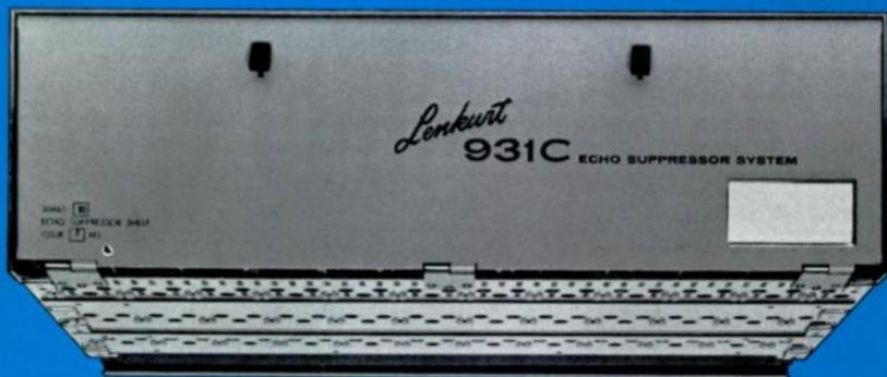
Lenkurt's 931C Echo Suppressor eliminates the echo encountered in satellite, transoceanic, and transcontinental circuits. This compact unit features microelectronic design and reliable printed circuit construction. For additional information, write Lenkurt, Dept. C134.
