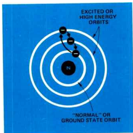
Figure 1. Pumping energy into an atom stimulates its electrons into higher energy levels. As they return to their "normal" state, this energy is emitted in the form of photons. More electrons available at the second level improves laser action.
