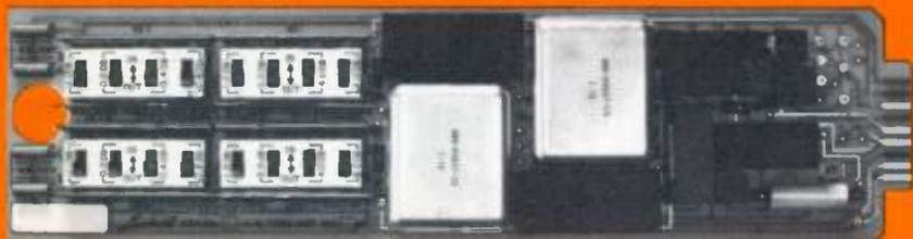
LENKURT'S 5540A FOUR-WIRE TERMINATING UNIT has eliminated the traditional use of separate pads or strappable terminals for attenuation adjustments between four-wire facilities and two-wire office equipment. Other advantages of the 5540A include improved performance, low cost, compact size, and front-access test points. For more information, write Lenkurt, Department C134.
