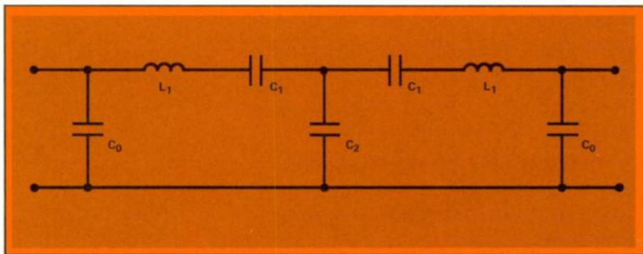
Figure 6. By knowing the values of the four electrical components illustrated, the equivalent two resonator crystal can be designed.
