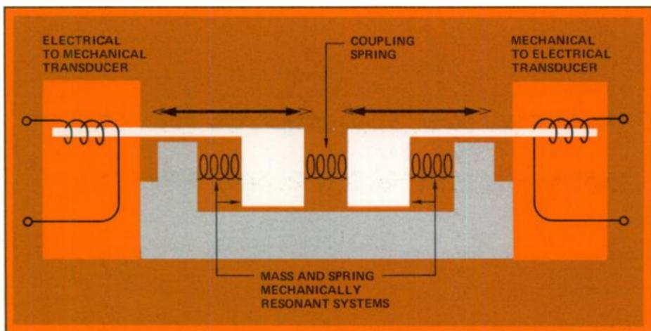
Figure 2. A mechanical model can be used to explain acoustically coupled crystal resonators.
