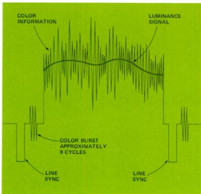
*Figure 1. The composite video signal. The color burst is transmitted during the blanking pulse to serve as a phase reference for the color information which modulates the basic video or luminance signal.*
