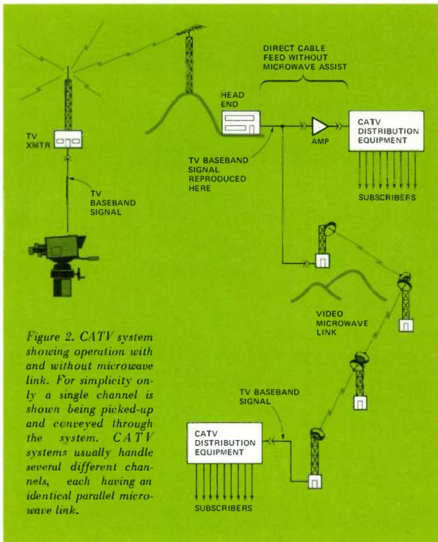
Figure 2. CATV system showing operation with and without microwave link. For simplicity only a single channel is shown being picked-up and conveyed through the system. CATV systems usually handle several different channels, each having an identical parallel microwave link.
