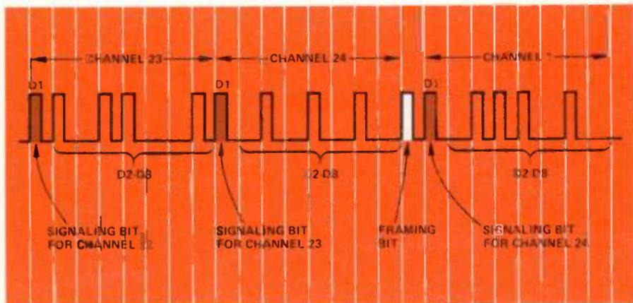
Figure 1. Frame format of D1 channel bank consists of 24 8-bit PCM words plus one framing time slot. The D1 time slot in each word is reserved for signaling information for the previous channel.
