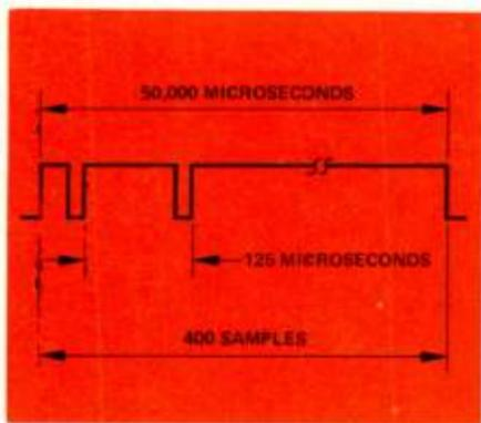
Figure 3. Each dial pulse is sampled approximately 400 times at an 8-kHz sampling rate.
