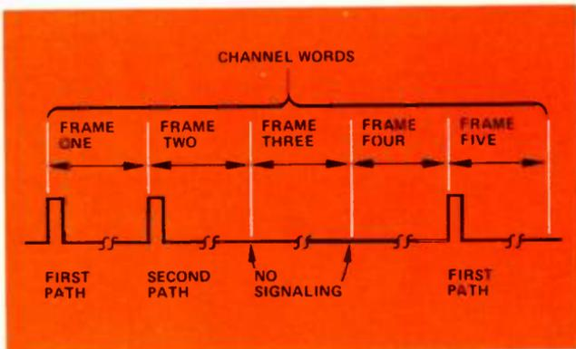
be avoided with a different technique for providing two signaling paths. This improved two-path arrangement is referred to as D1B.
