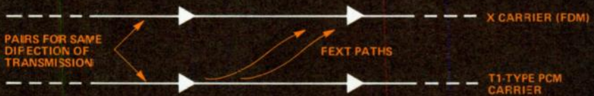
Figure 2B. Far-end crosstalk (FEXT) from T1-type carrier to X carrier.
