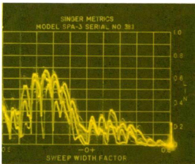
Figures 5 and 6 show the power spectrum of the line signal as it appears at the output of a PCM terminal under different traffic conditions. These photographs were taken in the field on a working 24-channel DIA system. Figure 6 shows that the power spectrum only *approaches* a spectral line condition due to the presence of
