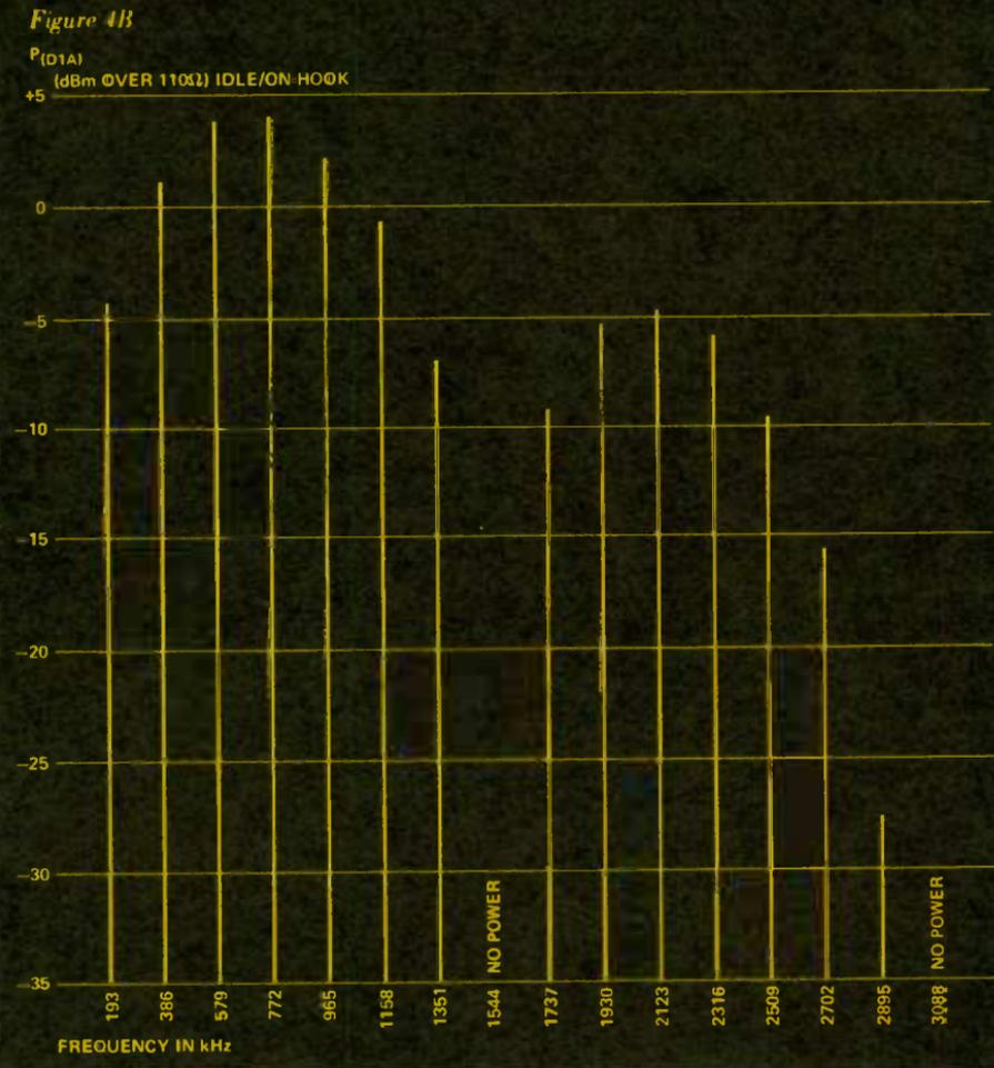
Figure 4A shows the pulse pattern as it appears out of a PCM terminal or regenerator in the idle/on-hook condition when D1A (D1/D8) signaling is used. The resulting line power spectrum is shown in Figure 4B.
