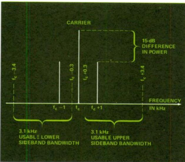
Figure 4. When a carrier of frequency  $f_c$  is modulated by a sinusoidal 1-kHz test tone, sideband frequencies appear at frequencies  $(f_c - 1)$  kHz and  $(f_c + 1)$  kHz. Each one of these two sideband frequency components are of a power level 15 dB below the level of the carrier. This is based on the test tone modulating the carrier with a modulation index of 0.35 (such as in a non-companded 47A system).
