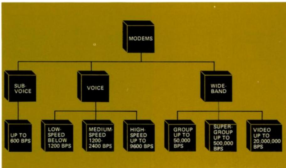
Figure 6. Bandwidth and transmission speed are generally related as shown in this chart – the wider the bandwidth, the higher the speed.
