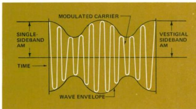
Figure 4. The wave envelope is the same as the modulating data signal. The bandwidth of the double-sideband AM signal is twice the bandwidth of the modulating signal.
