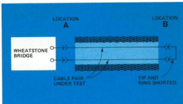
Figure 11B. Conductor resistance balance measurements.
