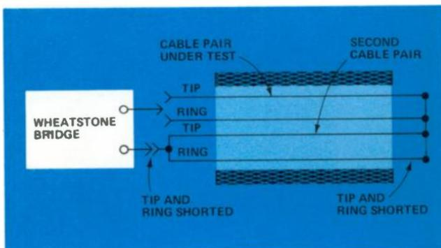
To measure the conductor resistance balance, the Wheatstone bridge should be connected as shown in Figure 11B, using a second pair in the same cable as a third conductor. Individual measurement of the tip and ring conductors of the pair under test is necessary and is performed as shown by the arrow connections. First the tip then the ring of the pair under test is measured using the second cable pair as a return path.
