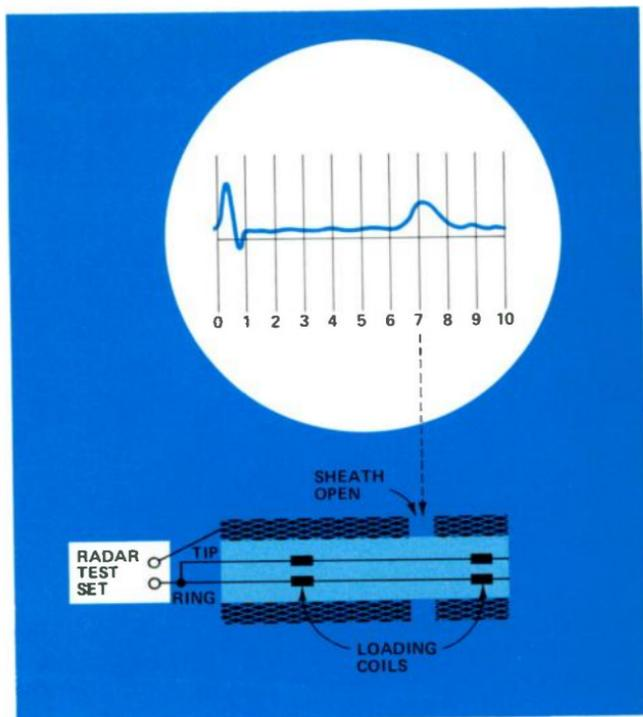
water, or earth conductivity is low (40 to 50 ohms), the capacitance tends to become more constant, and a pulse may be returned with sufficient strength to be visible. Figure 4 shows the grounded sheath oscilloscope display with the corresponding test set connections.
