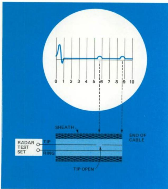
*Figure 1A. A pair with one conductor open will show a positive return pulse.*
