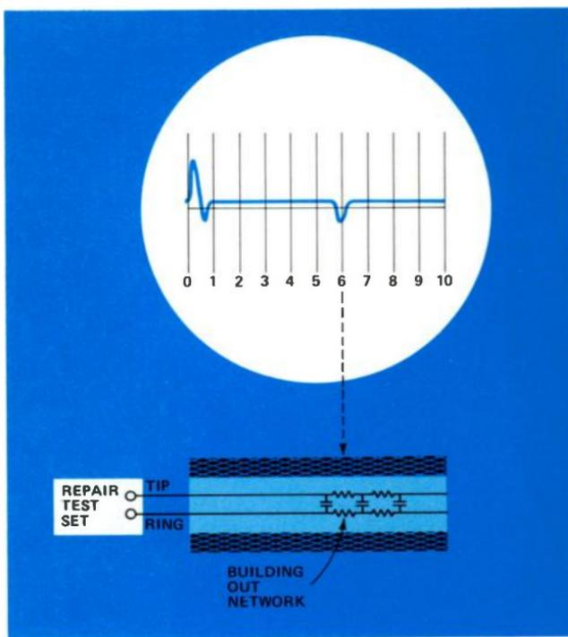
line and will give a negative pip similar to that of a bridged tap, but of lesser amplitude. The propagation velocity constant varies by approximately 1% per gauge number. (A change from 22 to 24 gauge will change the PVC by about 2%.)
