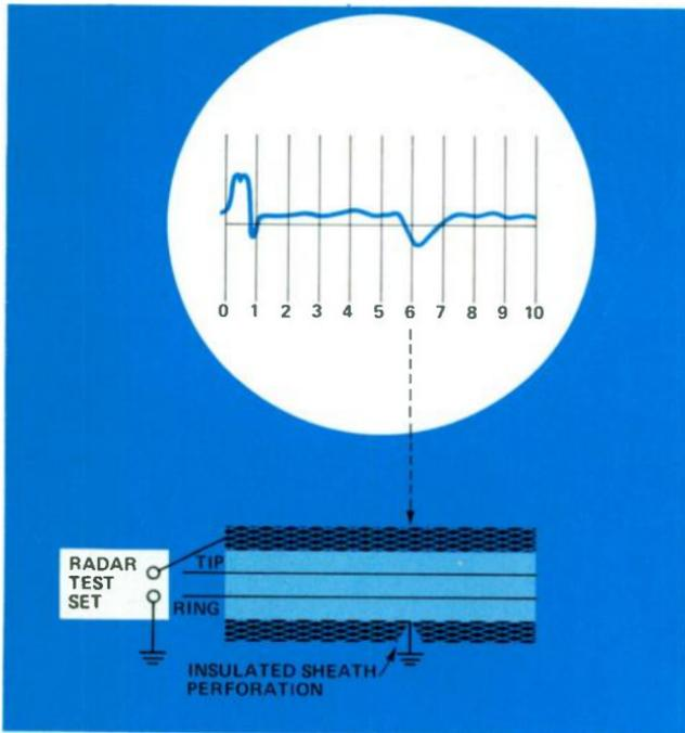
Figure 4. Grounded sheath on buried cable.
