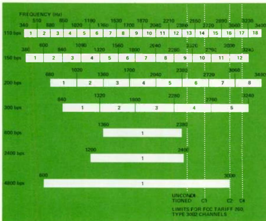
Figure 1. Data channel allocations and the necessary voice channel conditioning can be seen from this chart.
