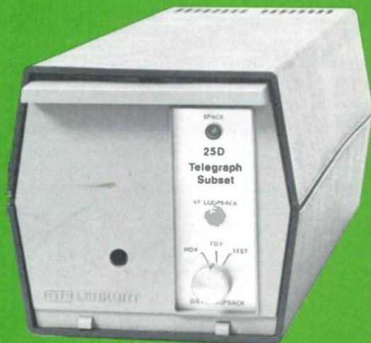
... is a compact, low-cost telegraph transmission system designed for multi-station, point-to-point, and switched network applications at speeds of 75, 110, 150, and 200 bauds.
