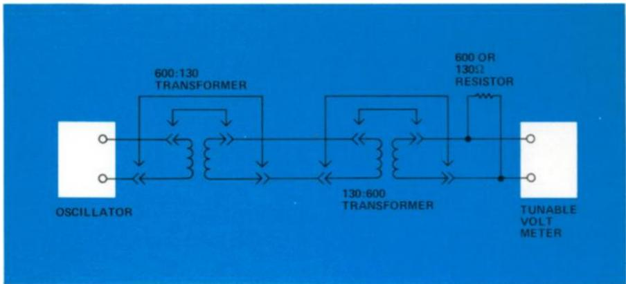
Figure 13A. Equipment arrangement for calibration.
