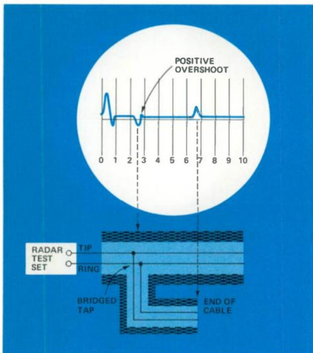
Figure 7. Bridged taps appear as negative pips with a positive overshoot.
