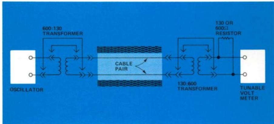
Figure 13B. Equipment arrangement for cable frequency-attenuation test.
