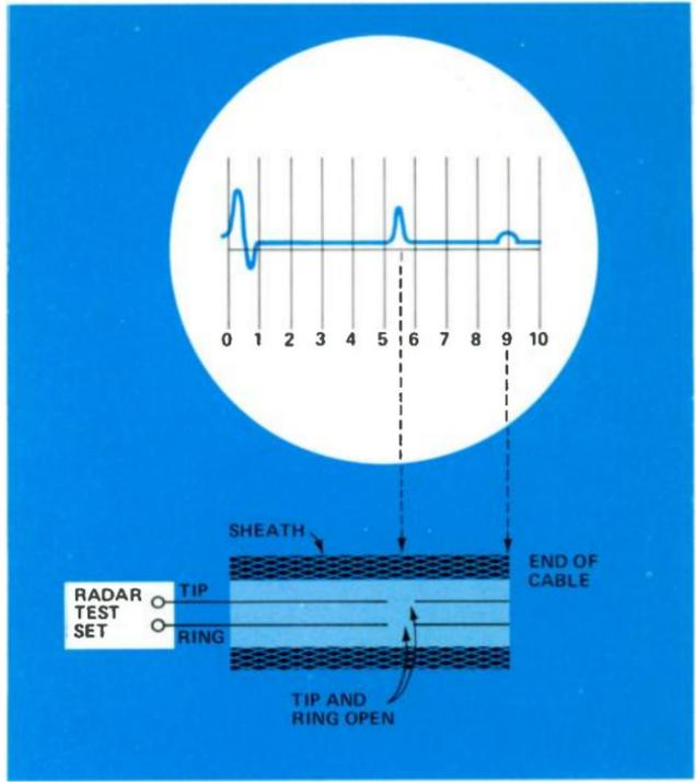
a 26-gauge conductor, the maximum fault location distance is about 4000 feet. For greater distances (8000 to 10,000 feet) a special pulse amplifier must be used to see the return signal.
