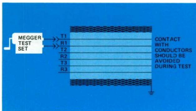
Figure 12A. Megger test on one cable pair.
