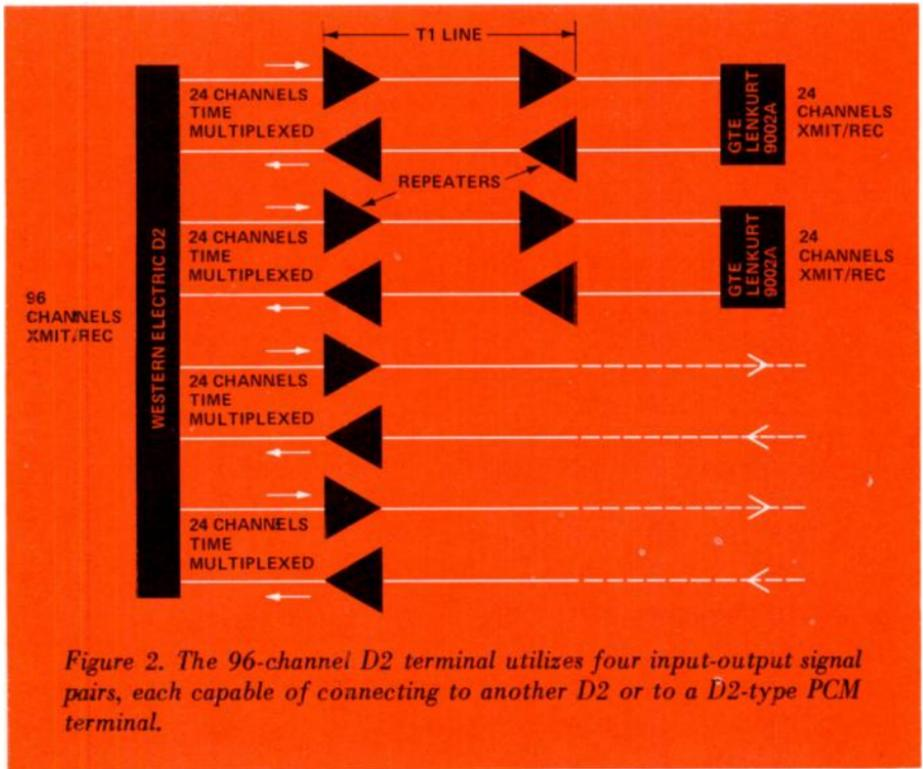
Figure 2. The 96-channel D2 terminal utilizes four input-output signal pairs, each capable of connecting to another D2 or to a D2-type PCM terminal.
