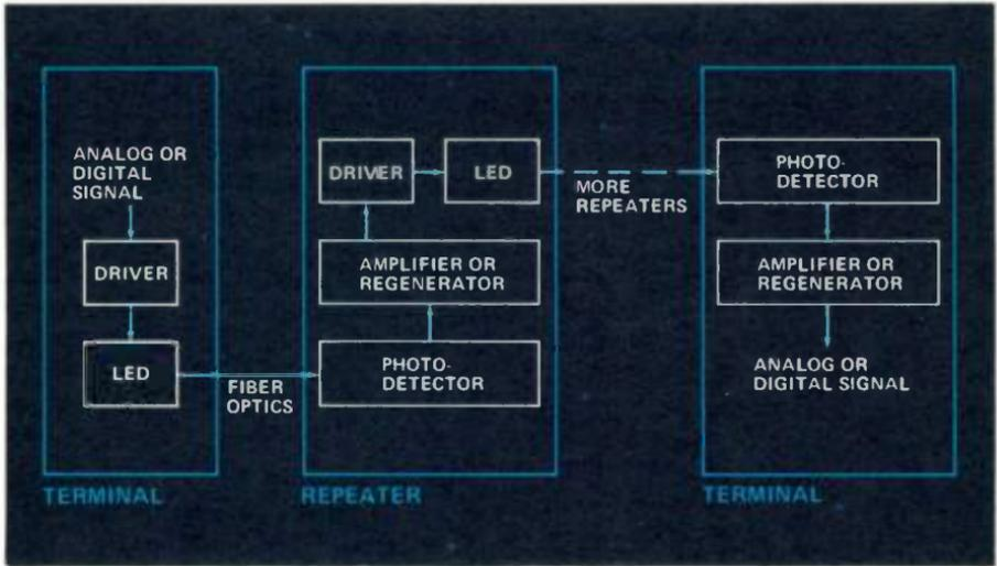
Figure 3. A simple optical transmission system can be designed for analog or digital signals using LED's as the light source.
