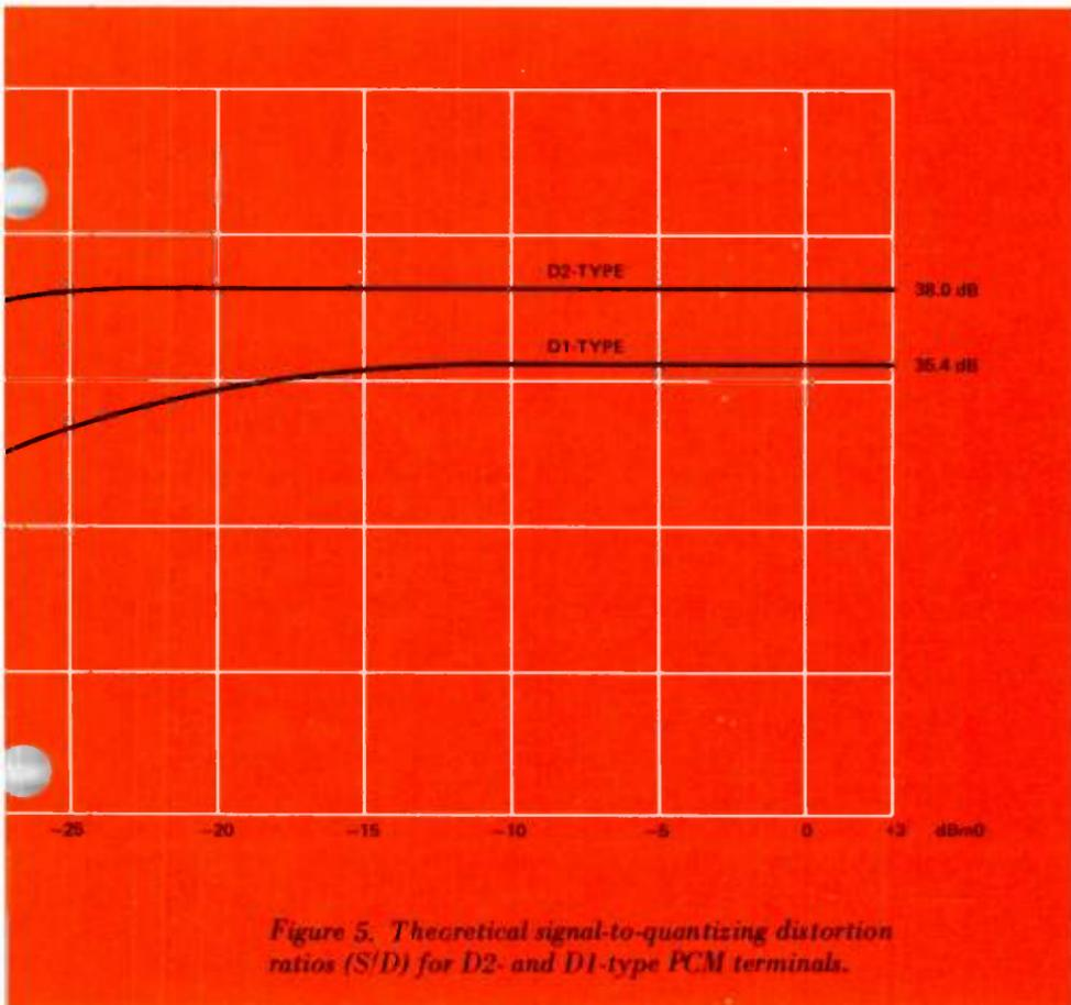
Figure 5. Theoretical signal-to-quantizing distortion ratios (S/D) for D2- and D1-type PCM terminals.
