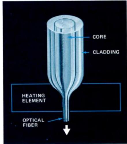
Figure 2. Fiber optics can be made from a glass rod placed inside a glass cylinder of a lower index of refraction.
