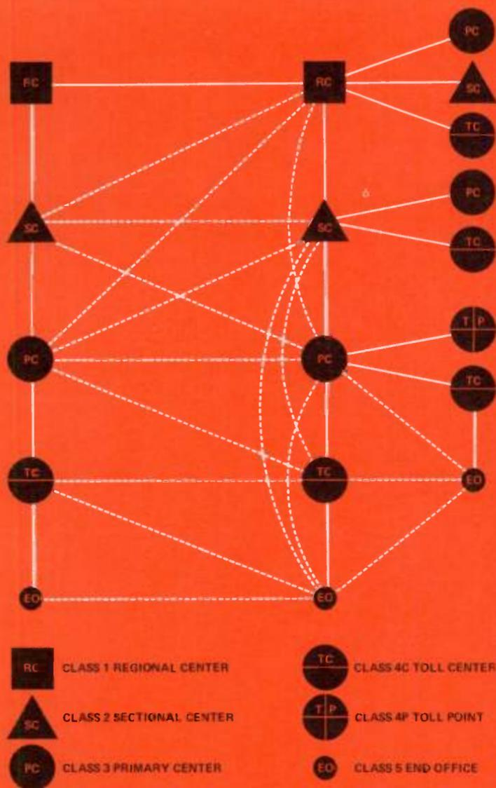
Figure 1. Hierarchical structure of the telephone switching network in the United States. Solid lines indicate main lines of connection within the hierarchy; dashed lines show examples of so-called "high-usage trunks" that can be connected between any two offices (regardless of rank) whenever the traffic volume justifies it.
