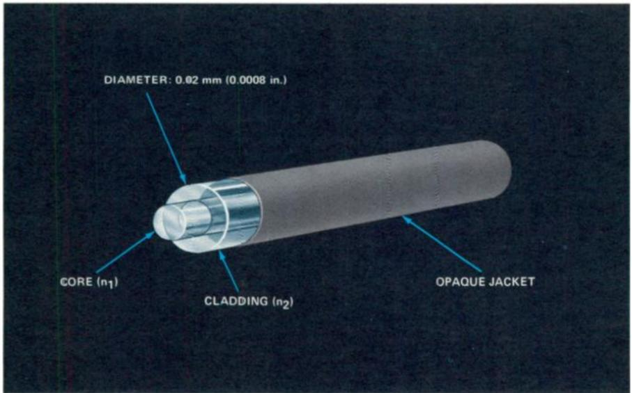
*Figure 1. The index of refraction of the fiber optical core ( $n_1$ ) is greater than the index of the cladding ( $n_2$ ). An opaque material can be placed around the fiber, like a jacket, to eliminate crosstalk between adjacent fibers.*
