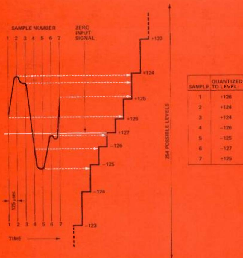
Figure 3. In a D2-type terminal, each voltage sample is quantized to one of 254 possible levels.
