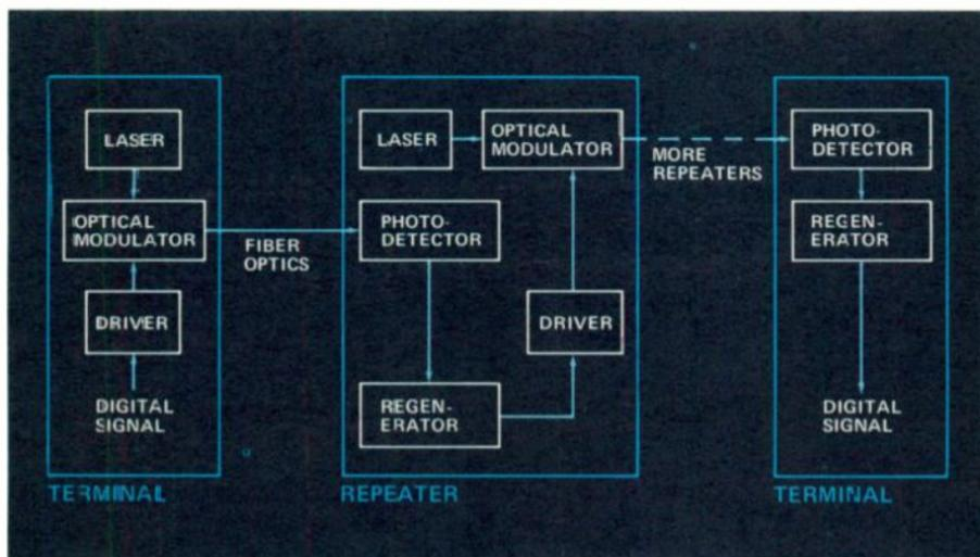
Figure 4. Transmission systems using non-injection laser sources have wider bandwidths than those using injection light sources and are quite suitable for digital transmission, especially PCM.
