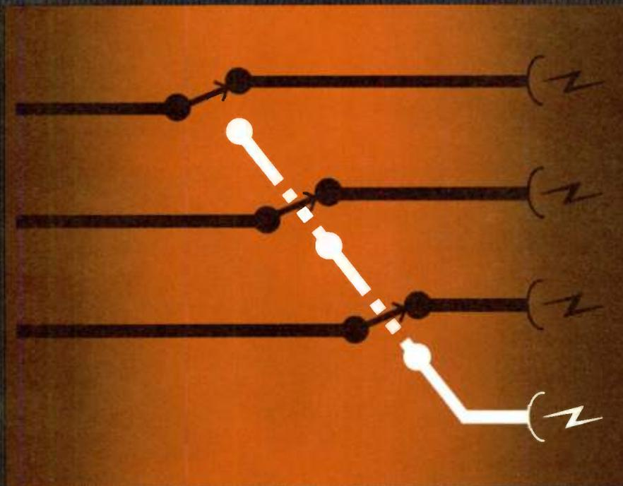
A multiline switching system provides protection for microwave transmission paths. It is not only an economical method of protection, but is also a means of conserving bandwidth in crowded microwave bands.
