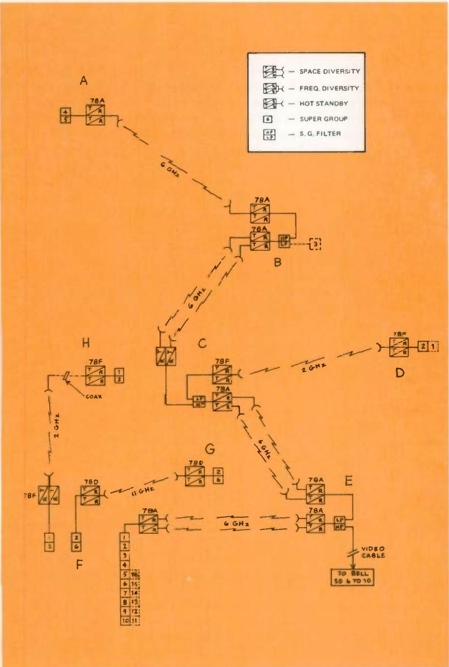
Figure 2. In laying out a microwave system, a block diagram is prepared showing all the required repeater stations.
