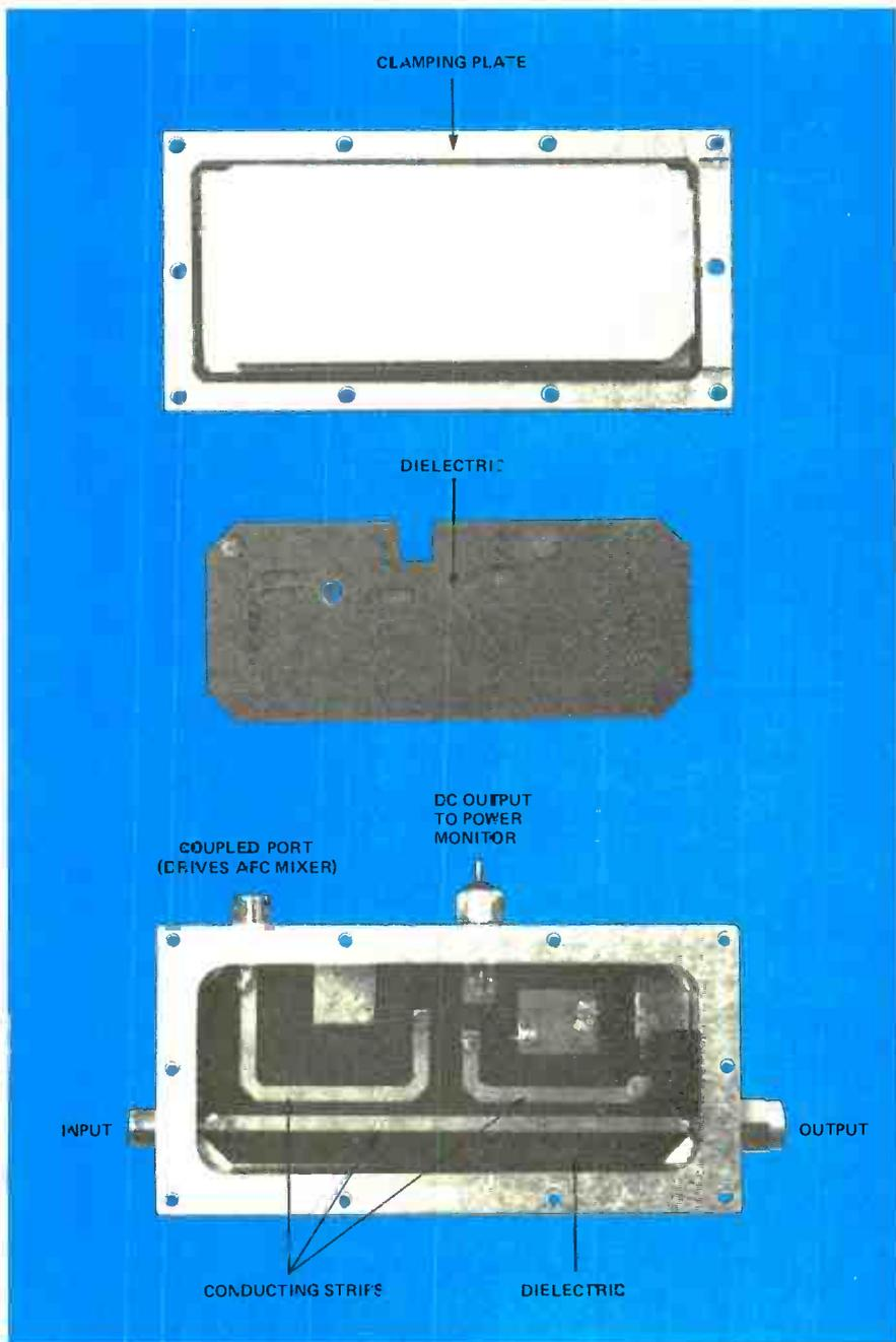
Figure 8. The principle of the strip line is used in construction of directional couplers.
