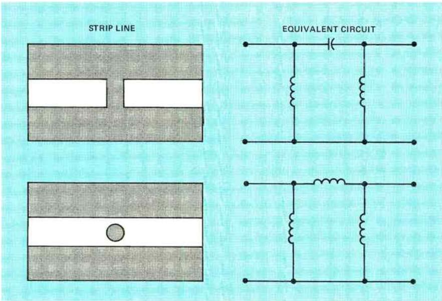
Figure 7. A space or circle positioned along a strip line gives the equivalent circuit of networks made up of discrete components.
