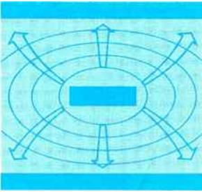
The transmission line is an important component of any microwave transmission equipment. Within a certain frequency spectrum, strip transmission line provides an efficient and compact conveyance for microwave signals.
