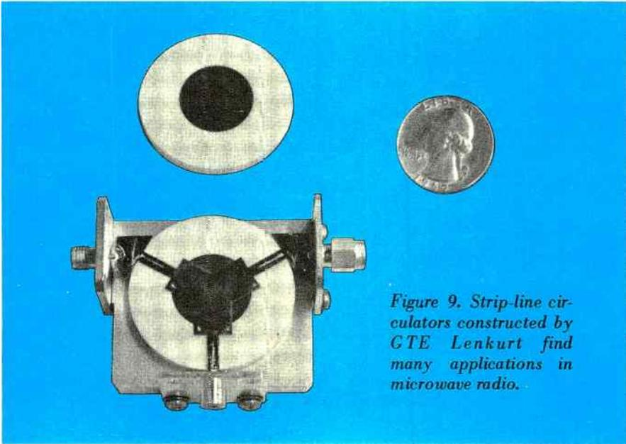
*Figure 9. Strip-line circulators constructed by GTE Lenkurt find many applications in microwave radio.*
