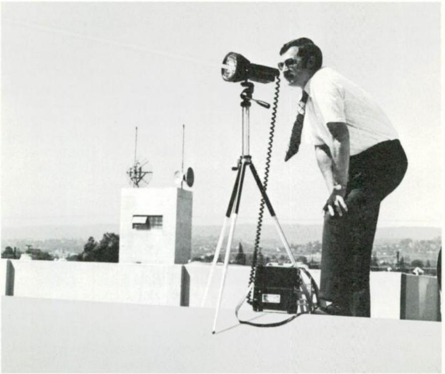
*Figure 4. A searchlight provides an efficient method of “flashing” a path in daylight and poor visibility at distances up to 30 miles.*
