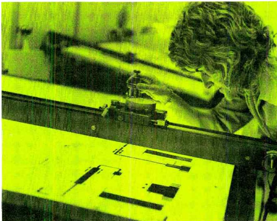
*Figure 3. The first step in the construction of a microstrip circuit is the drawing of the dimensional pattern at ten times its normal size.*
