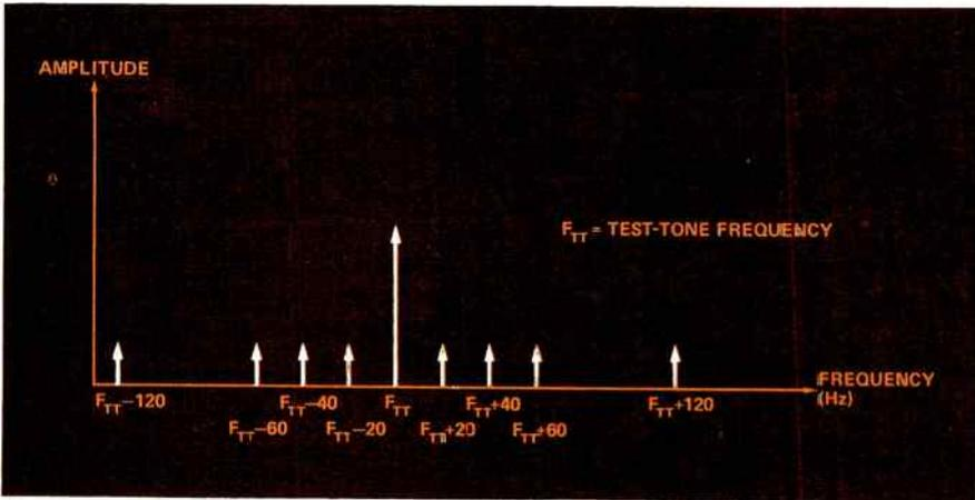
Figure 3. Phase jitter caused by power-line frequencies and telephone ringing frequencies have a definite spectral distribution.
