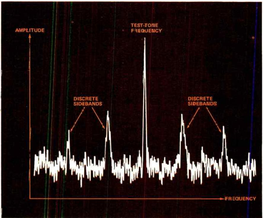
Figure 1. When testing for phase jitter, a single-frequency test-tone may appear to have a definite spectral distribution such as symmetric, discrete sidebands or it can have random, low-amplitude sidebands like noise.
