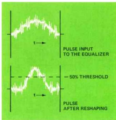
Figure 3. The reshaping function restores the correct pulse width to the incoming pulse.
