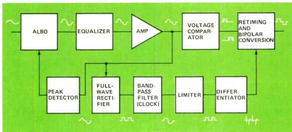
Figure 5. The digital pulse train supplies its own timing information.
