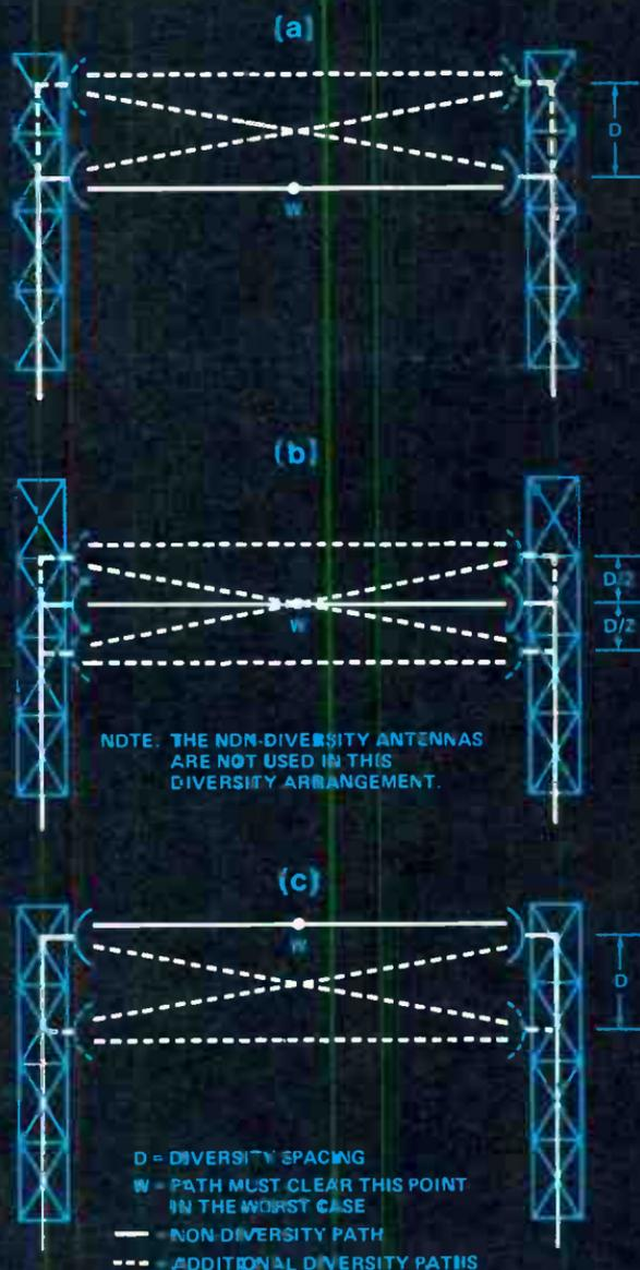
Figure 2. In the most conservative space diversity arrangement (a) with all the spacing above the existing antenna, all paths give adequate clearance; when the spacing is split above and below the existing antenna (b), three out of four paths are good; and when all the spacing is below (c), only the top-to-top path is good.
