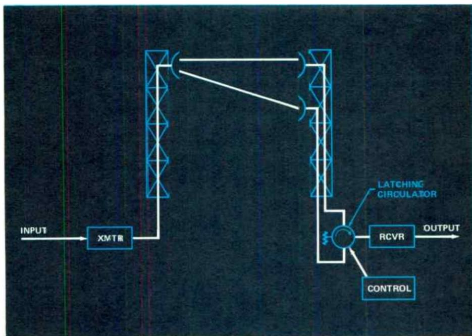
Figure 5. Space diversity without equipment redundancy can also be done using a latching circulator for "blind" RF switching at the receiver.
