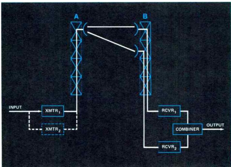
Figure 3. A one-way space-diversity systems uses diversity at the receiver end.
