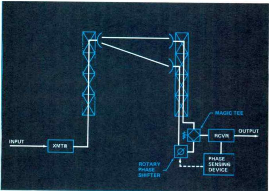
Figure 4. Space diversity without equipment redundancy uses a “magic Tee” for combining and a rotary phase shifter for automatic phase control.
