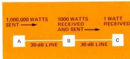
Figure 2. The expansion of a telegraph line necessitates an increase in power.
