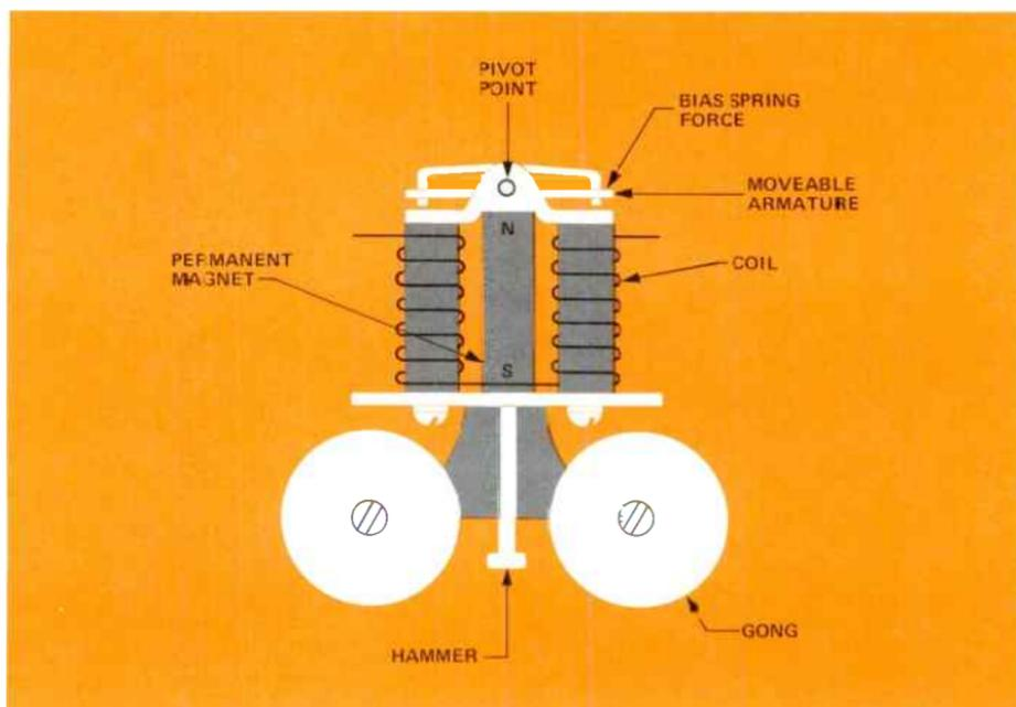
Figure 10. Typical telephone ringer arrangement.
